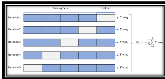
Figure 4.32: - Generalized working of K-Fold Cross Validation with k=5
