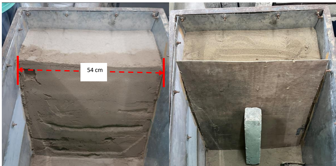
Fig.14 (Land slope constructed of 60° angle)
