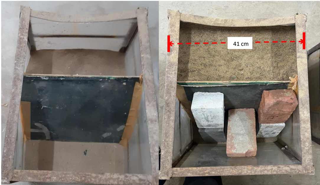
Fig.15 (Land slope constructed of 70° angle)
