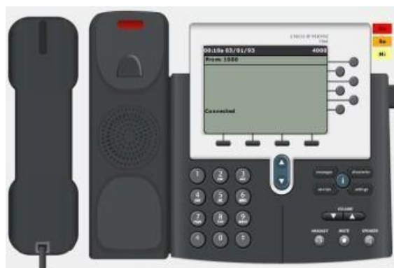
Fig. 8(b) User with number 4000 receives the call from user with number 1000. Connected message gets displayed on the screen.
