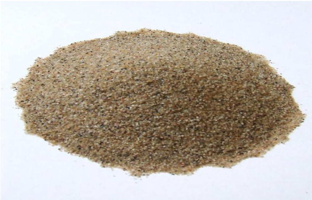
(fig.3) Fine Aggregates
