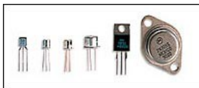
Typical transistor packages
