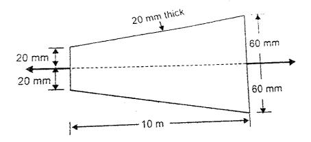
Q4. The steel rod ABC is attached to a rigid support and is unstressed at a temperature of  $25^{\circ}$ C. Temperature of both the portion is increased to  $150^{\circ}$ C. Knowing  $\alpha = 11.7 \times 10^{\circ}$  6/°C, E = 200 GPa. Find stress in both the portion of rod and deflection of point C.
