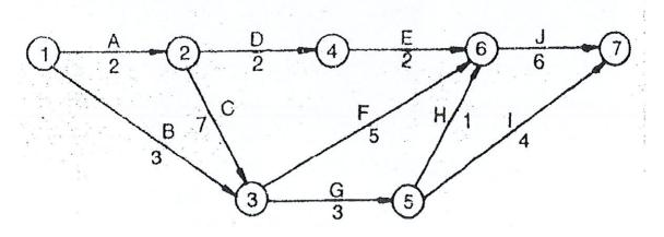
Q 3. From the given table below, find project's minimum cost and Optimum duration using graph paper
