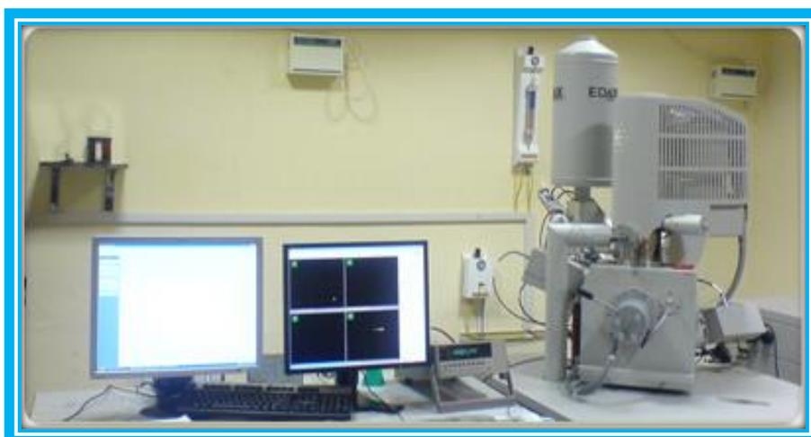
**Figure 2.8:** “FEI-Quanta FEG 200 HRSEM and EDX”
