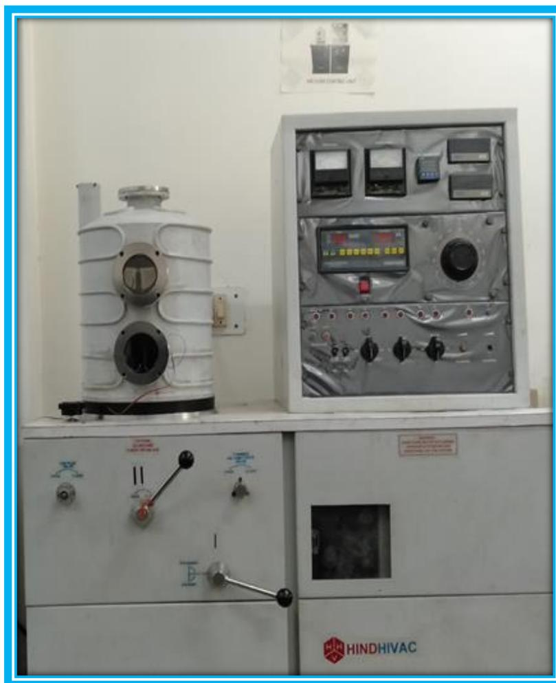
**Figure 2.5:** Vacuum coating unit HINDHIVAC
