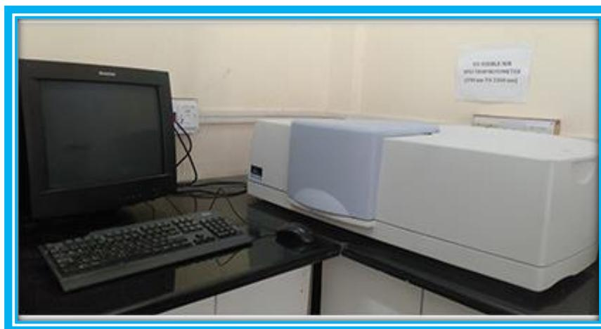
**Figure 2.9:** “Perkin Elmer Lambda 750 UV-visible-NIR spectrophotometer”
