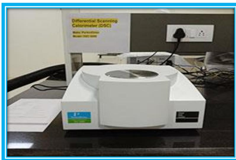
**Figure 2.12:** Perkin Elmer DSC system
