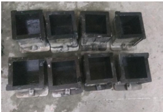
Fig. 1 Surface cleaned and oiled moulds
