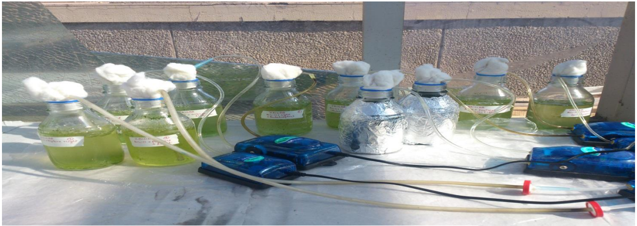
Fig. 18 Experimental setup for study of lipid induction in Chlorella sp.
