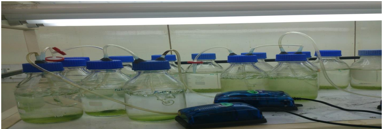
Fig.15 Experimental setup to study the growth kinetics of Chlorella sp.
