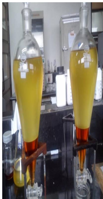
Fig.3 Separation of Biodiesel and its by-products in a separating funnel
