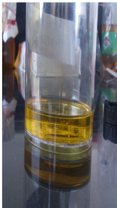
Fig.5 Biodiesel produced by two-step transesterification reaction. 45
