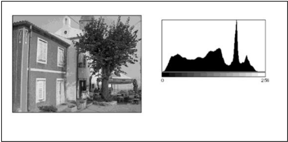
Figure 2.4: An 8 bit gray scale image and its histogram with 256 gray values
