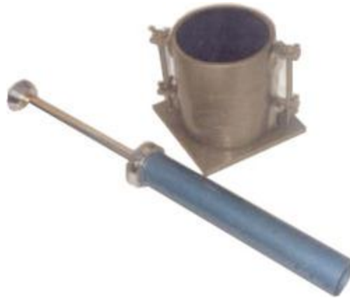
Wikipedia images of compaction test
