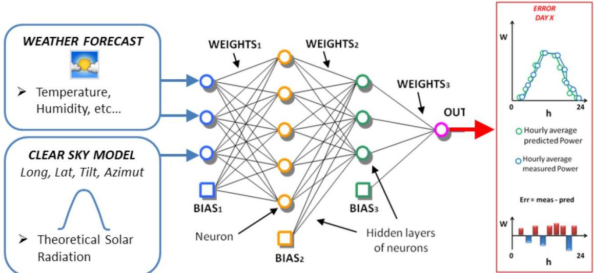
Figure 6.3: Diagrammatic representation of weather prediction using ANN.
