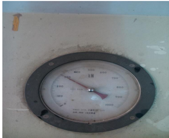
Fig. 6(b) : Compressive Strength Test Reading
