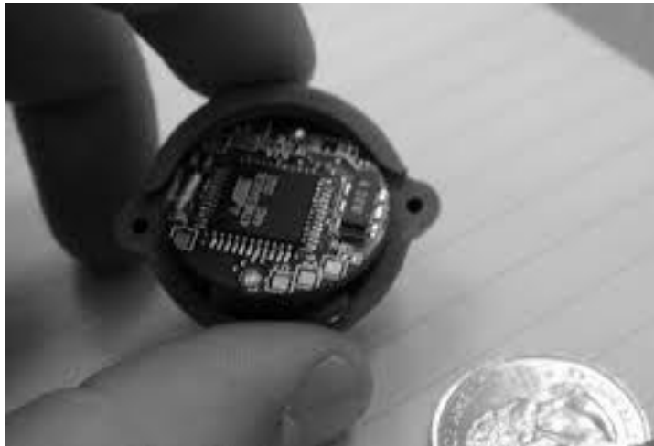
Figure 1.1.3 An illustration to show the size of a wireless network sensor node[Source: internet]
