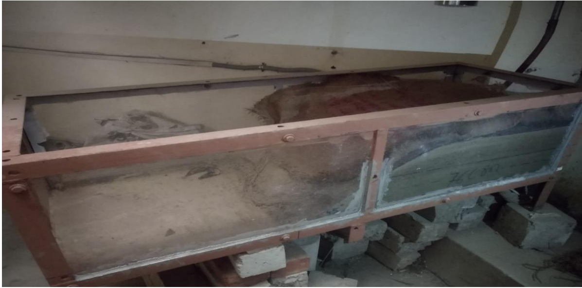
Fig 3.3.3: Steel box frame
