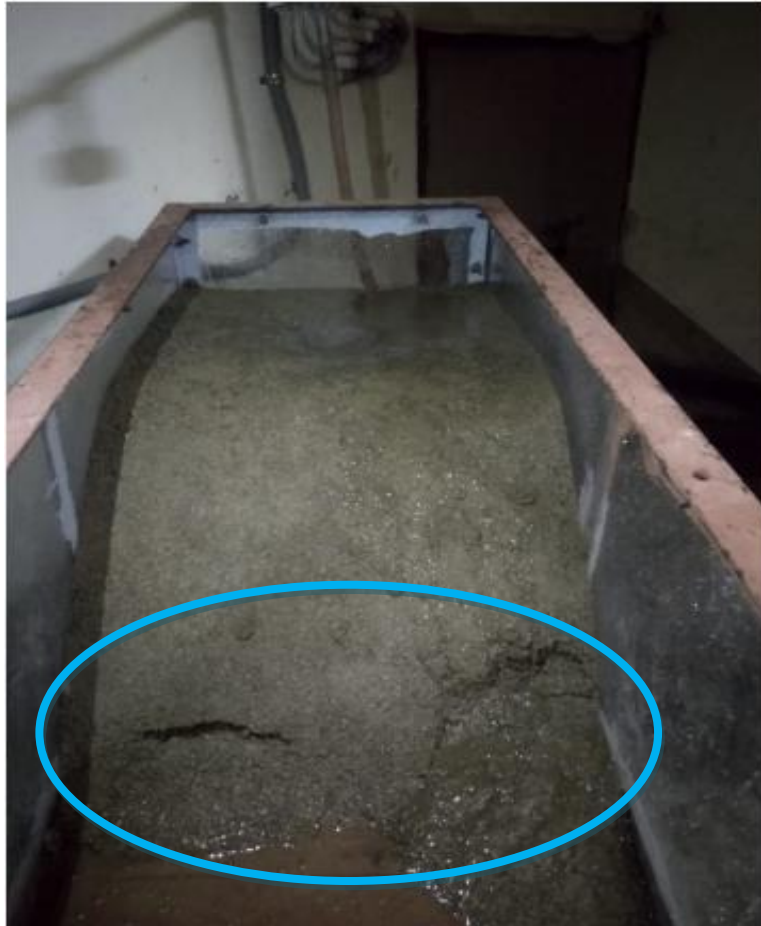
Fig 4.9.1: Slope failure and soil erosion without using jute mats
