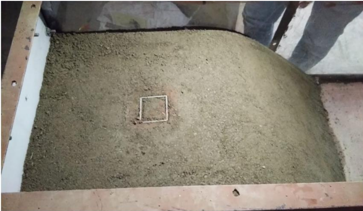
Fig 3.8 Calibration of field density in box model
