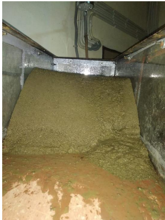
Fig 4.10: Slope failure and soil erosion at high intensity ( i=1.2\text{mm/hr} ) with using jute mats
