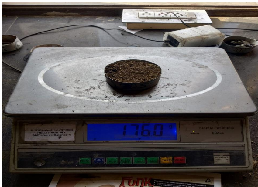
Fig 3.3.1: Water content determination
