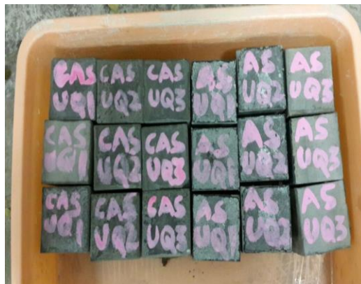
Figure 18 Blocks after Hot Water Curing
