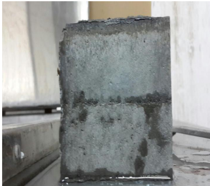
Figure 19 The block showing the separation of the particle into two layers due to over compaction
