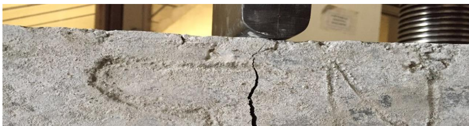
Figure 1 Flexure test on beam
