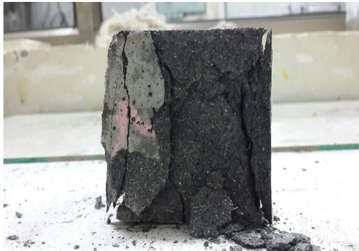
Figure 20 The failed block showing segregation of the material
