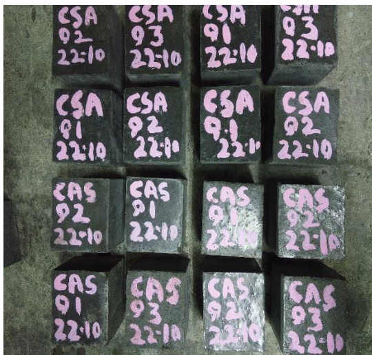
Figure 16 Blocks Before Hot Water Curing
