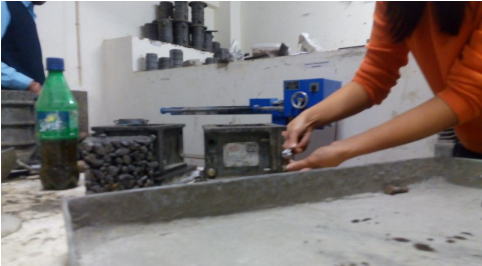
Figure 4.4 Demoulding of second trial pervious concrete.
