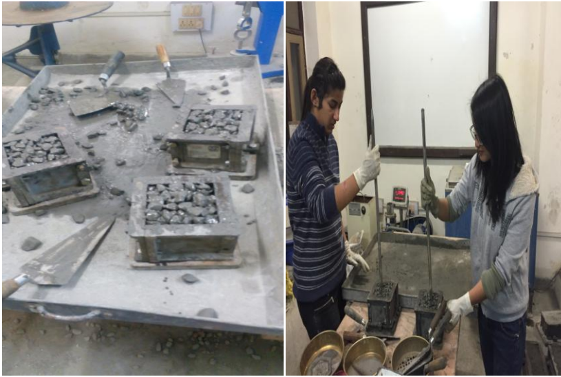
Figure 4.1 Three cubes casted in 10*10*10 cm mould according to first mix design
