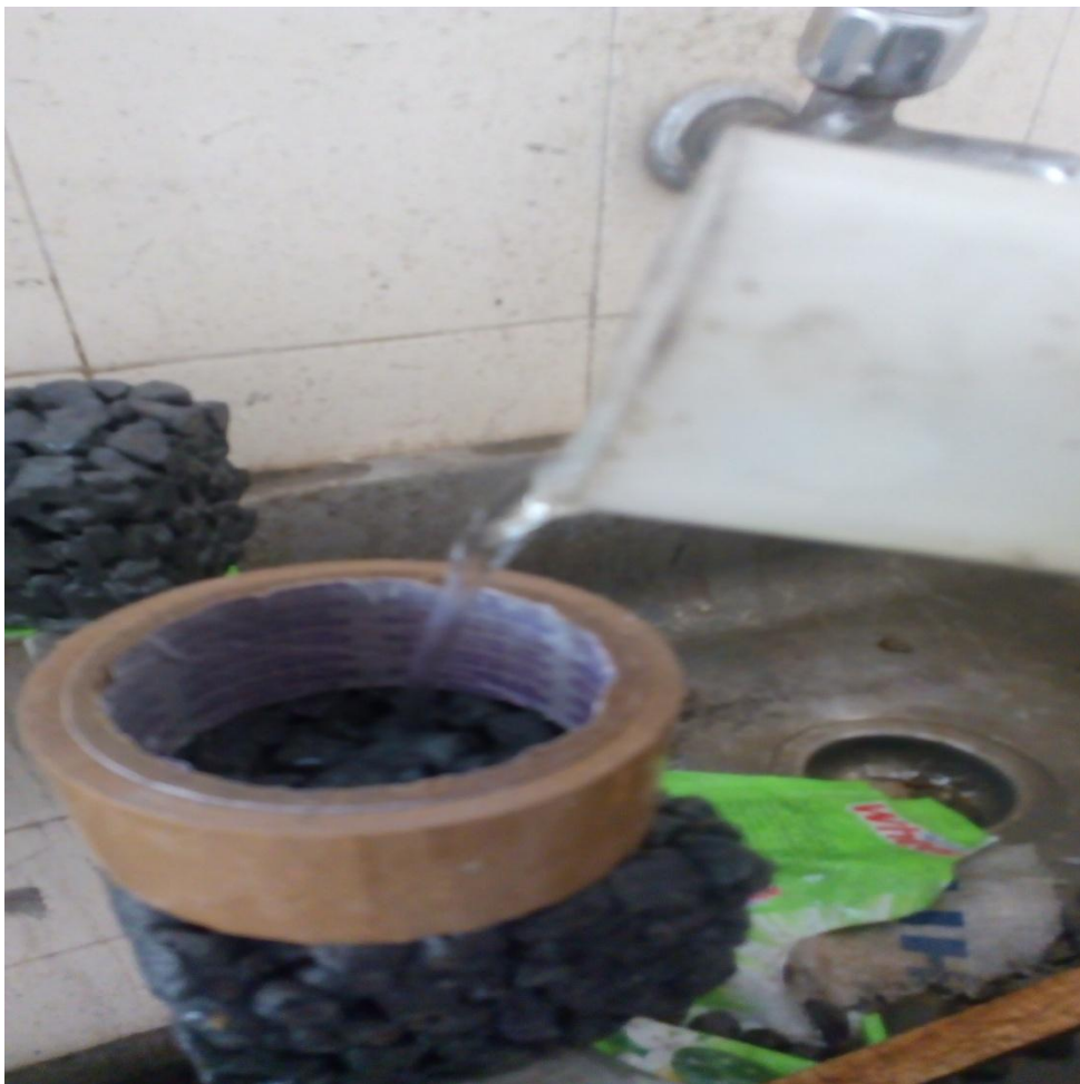
Fig 5.8 Infiltration test on Pervious concrete.
