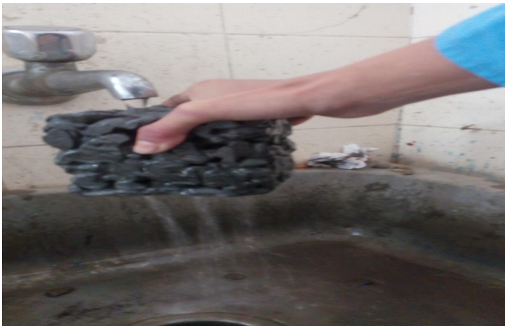
Figure 4.3 Water passing through first trial pervious concrete and checking its permeability.
