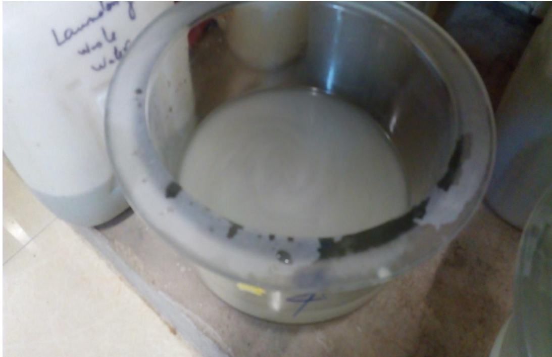
Figure 5.10 Acid solution after taking out the concrete cubes after 14 days.
