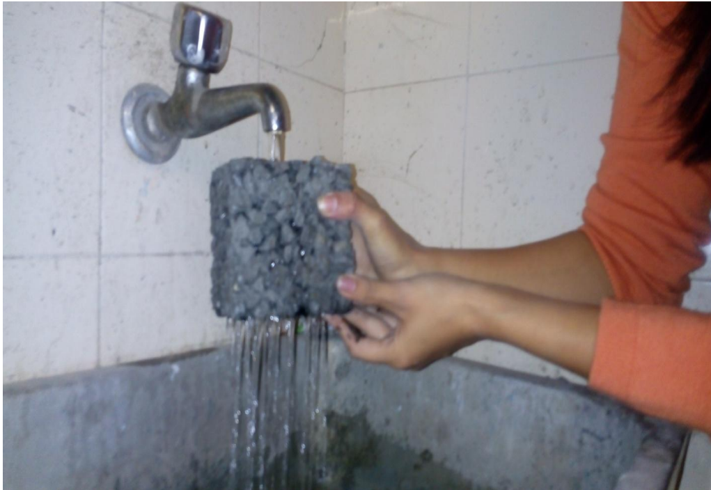
Figure 4.6 Second trial pervious concrete below the tap of water to check its permeability.
