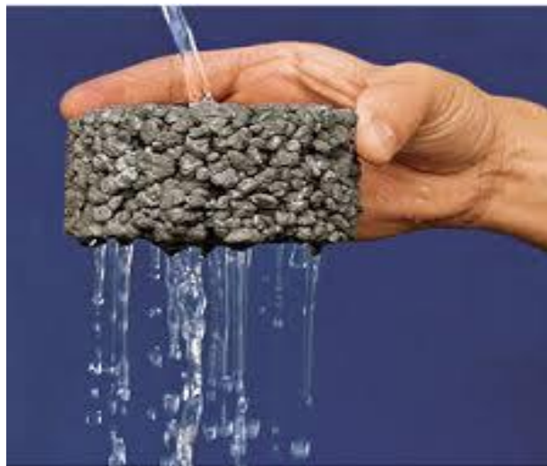
Figure 1.1 water passing through a Pervious concrete
