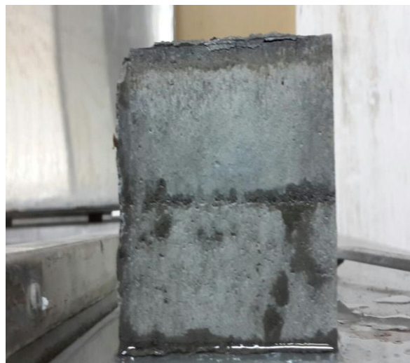
Figure 48: The block showing the separation of the particle into two layers due to over compaction
