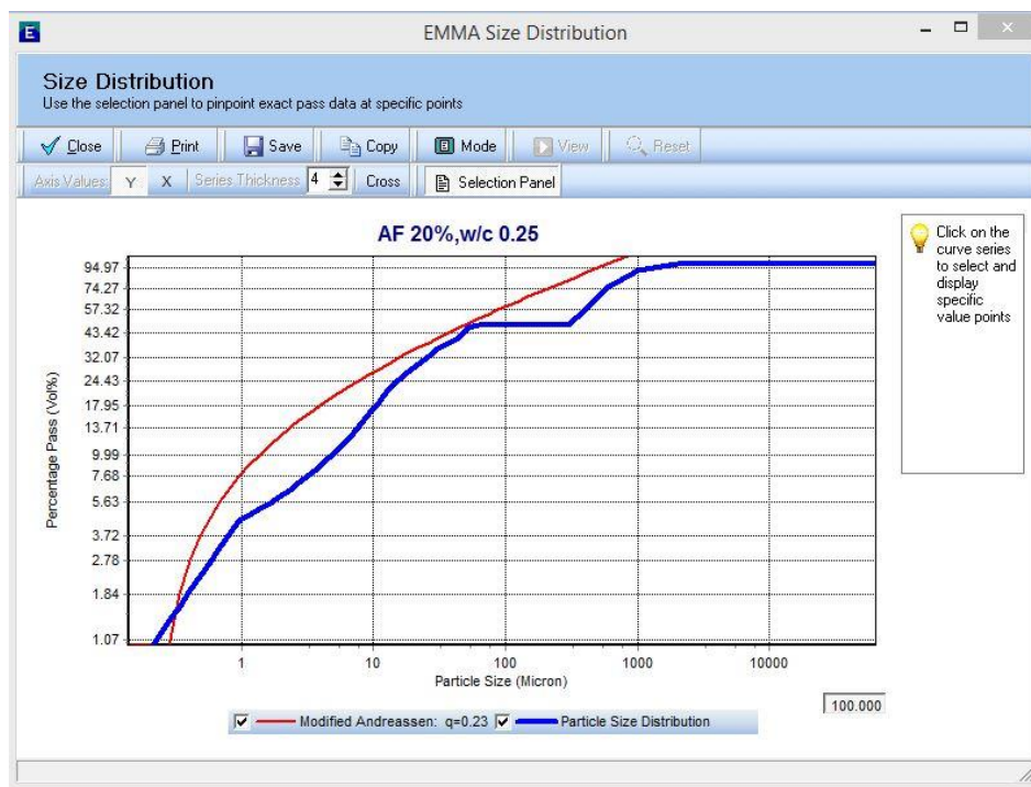
Figure 2: EMMA Analysis OPC 53 (80%) + Ultrafine slag (20%), w/c ratio=0.25
