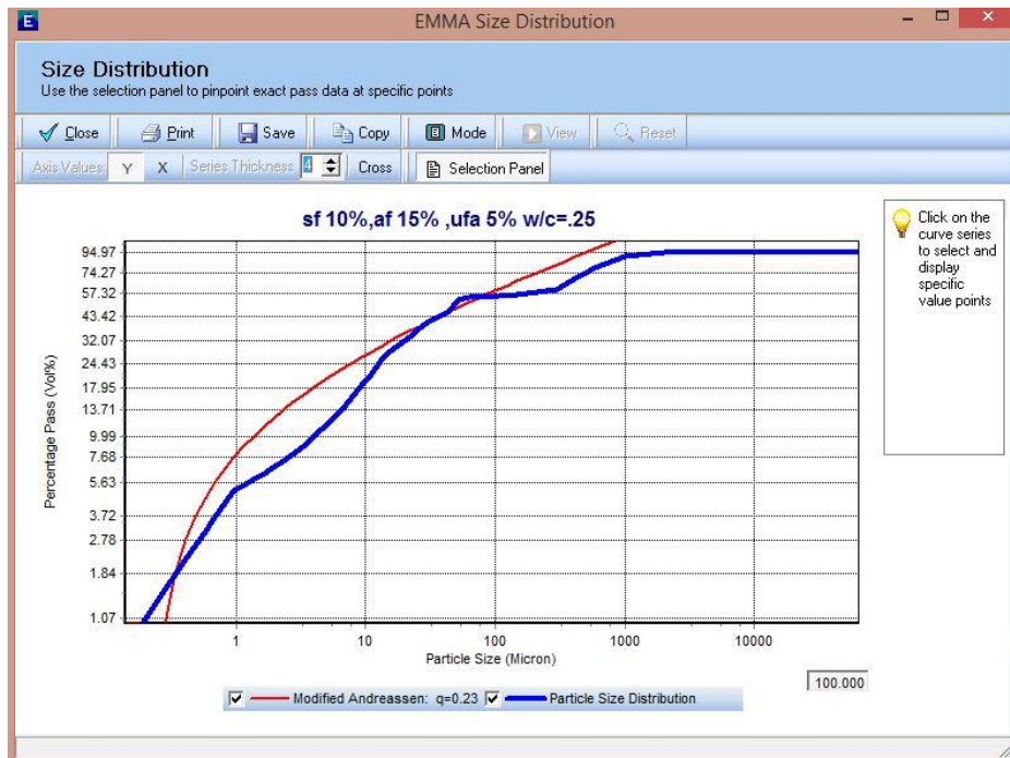
Figure 5: EMMA Analysis OPC 53 (70%) + Silica fume (10%) + Ultra-fine slag (15%) + Ultra-fine fly ash (5%), w/c ratio =0.25
