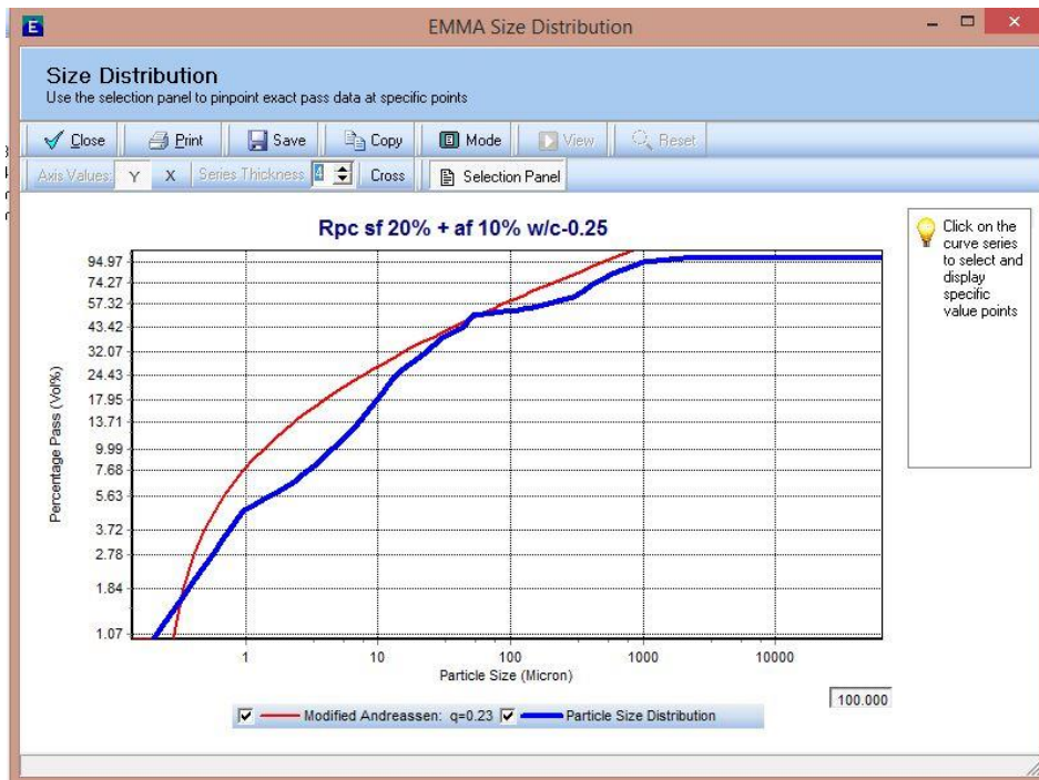
Figure 4: EMMA Analysis OPC 53 (70%) + Silica fume (10%) + Ultra-fine Slag (20%), w/c ratio=0.25
