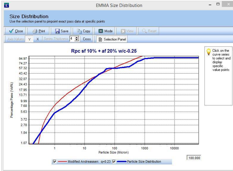
Figure 3: EMMA Analysis OPC 53 (70%) + Silica fume (10%) + Ultra-fine Slag (20%) w/c ratio=0.25
