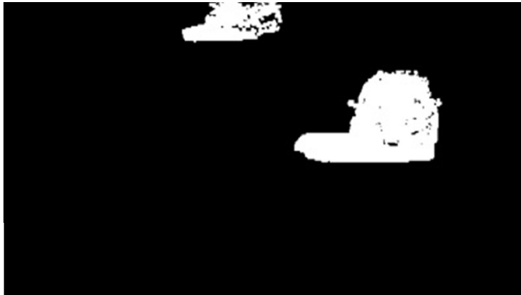
Fig 1.5: Moving cars are detected using blob analysis.
