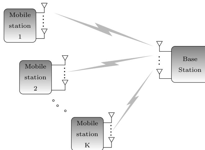
Figure 1.1: A typical wireless cellular uplink. (Courtesy of Singh, K. [6]).
