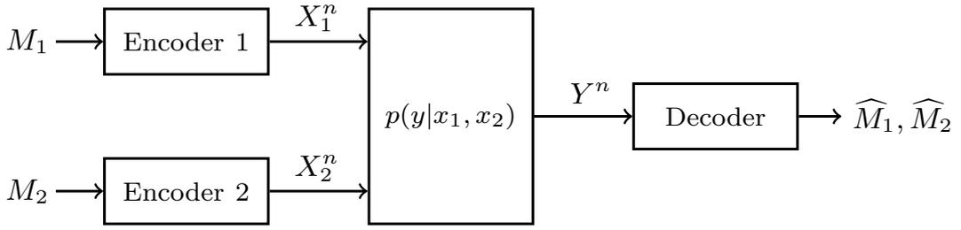
Figure 1.2: Two-User Discrete Memoryless Multiple access channel
