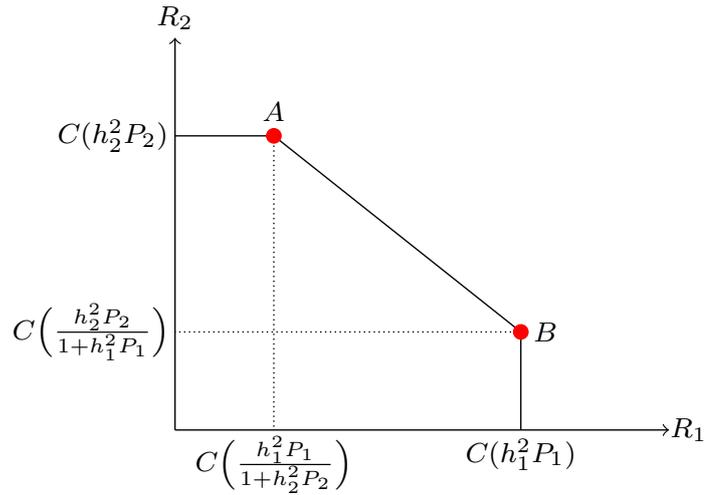
Figure 1.4: Capacity region of a Two-User Gaussian Multiple access channel
