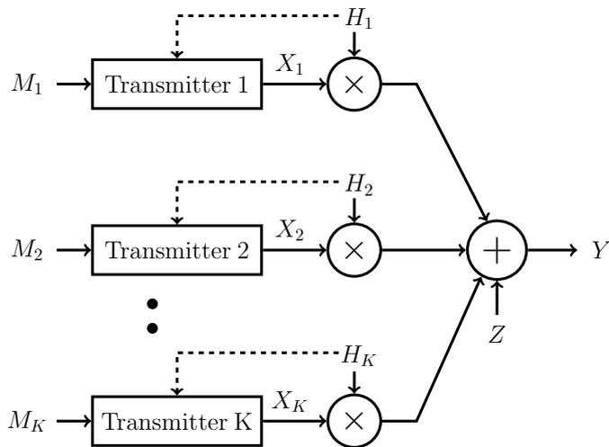
Figure 2.1: Decentralized/Distributed gaussian MAC. (Courtesy of Singh, K. [6])
