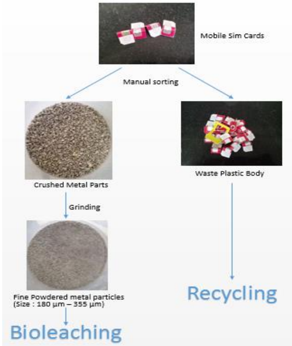
Figure 3.2: Physical treatment of obsolete mobile SIM cards pre 2 step Bioleaching experiment.
