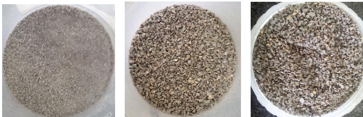
SIM particle size ~ 355 \mu m SIM particle size b/w 355-700 \mu m SIM particle size > 700 \mu m
