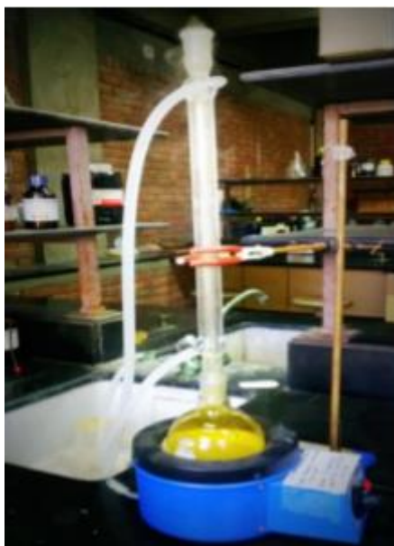
Figure 3.3: Acid digestion of e-waste using aqua regia.
