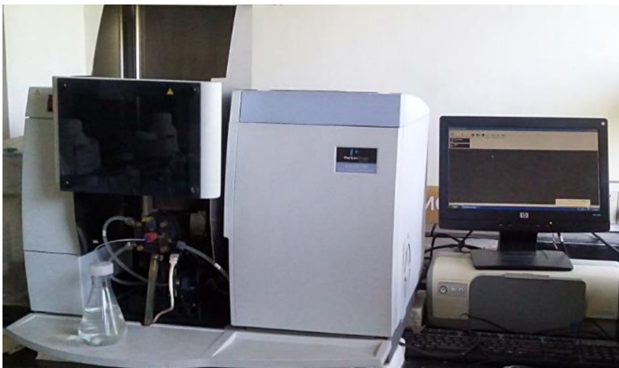
Figure 3.4: Perkin Elmer A Analyst 400 Atomic Absorption Spectrophotometer used for Analysis.
