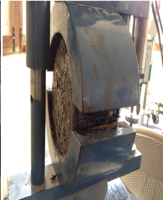
Fig 3.5(b) Sample placed in Marshall test apparatus
