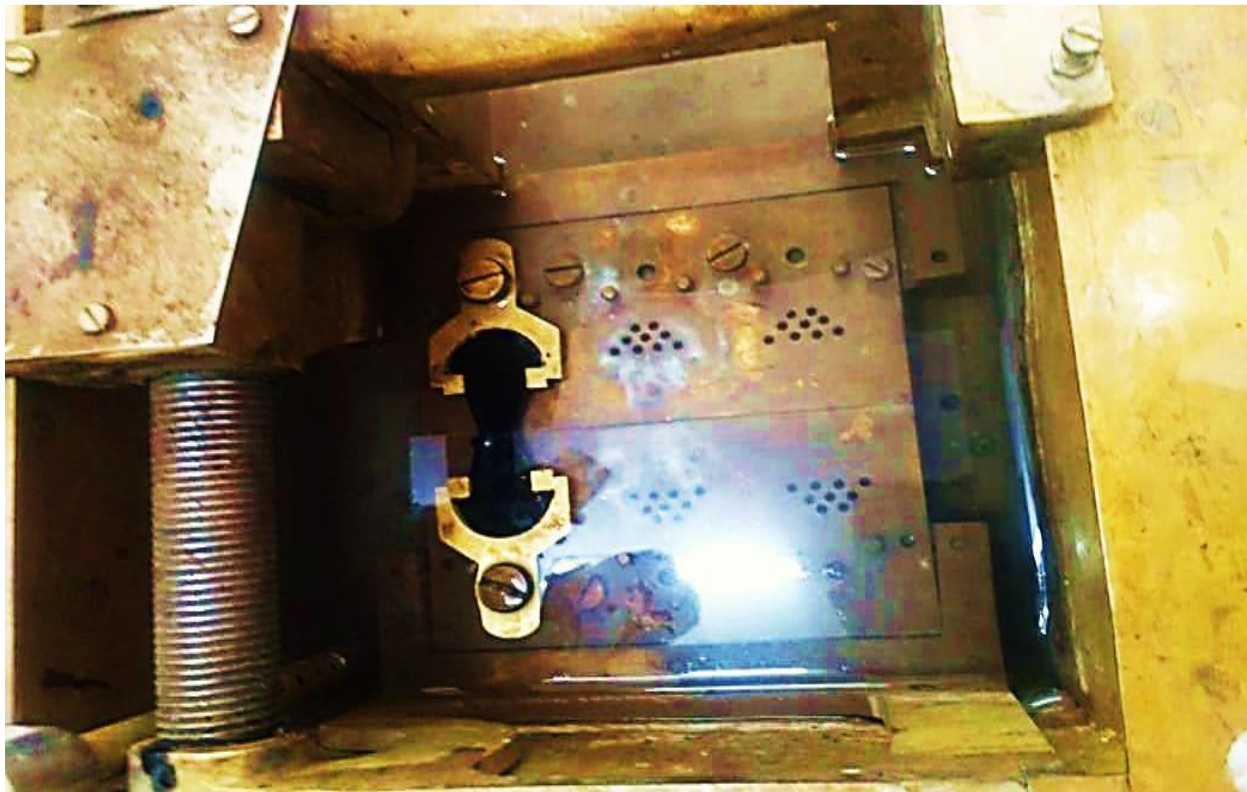
Fig 3.3 Ductility Test Apparatus
