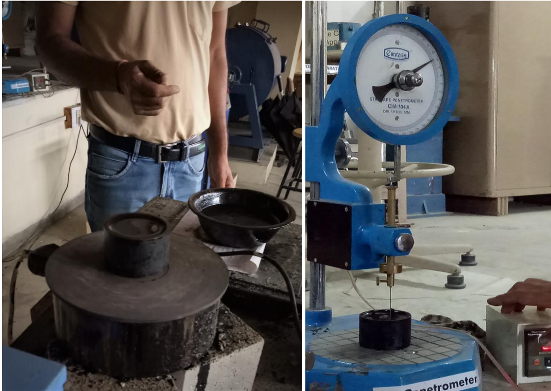
Fig 3.2 (a) Bitumen sample in mould
