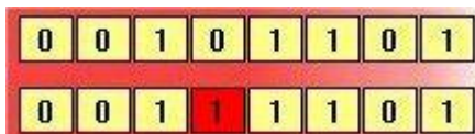
Figure3.15. Diagram showing the effect of mutation on an individual in a population of 8-bit strings where mutation occurs at position 4, changing the 0 at that position in its genome to a 1
