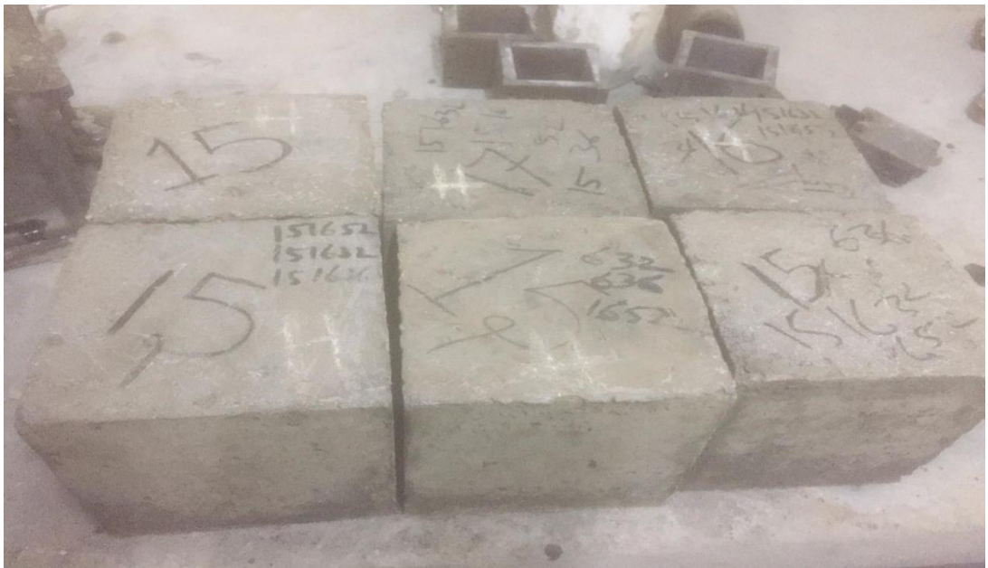
Figure 3.7 Demoulded marked concrete cubes before curing
