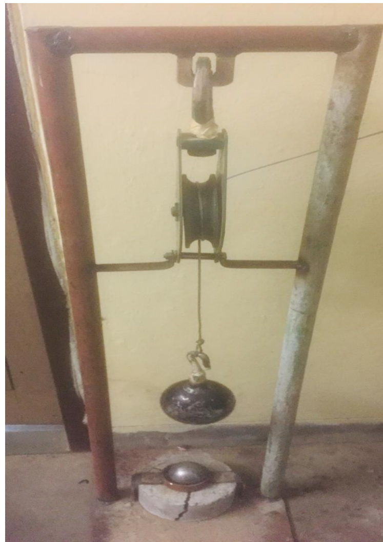
Figure 3.16 Drop weight test apparatus used for impact test
