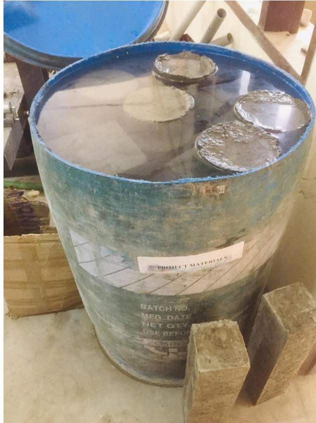
Figure 3.10 Concrete specimens placed for curing in curing tank
