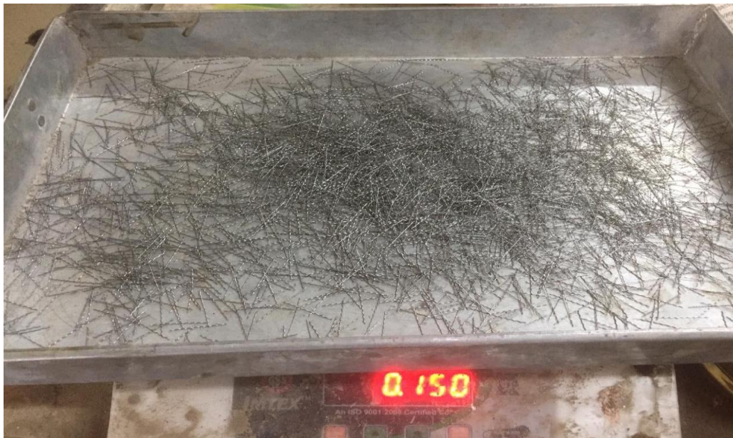
Figure 1.1 Steel fibre of length 30 mm and diameter 0.5 mm.
