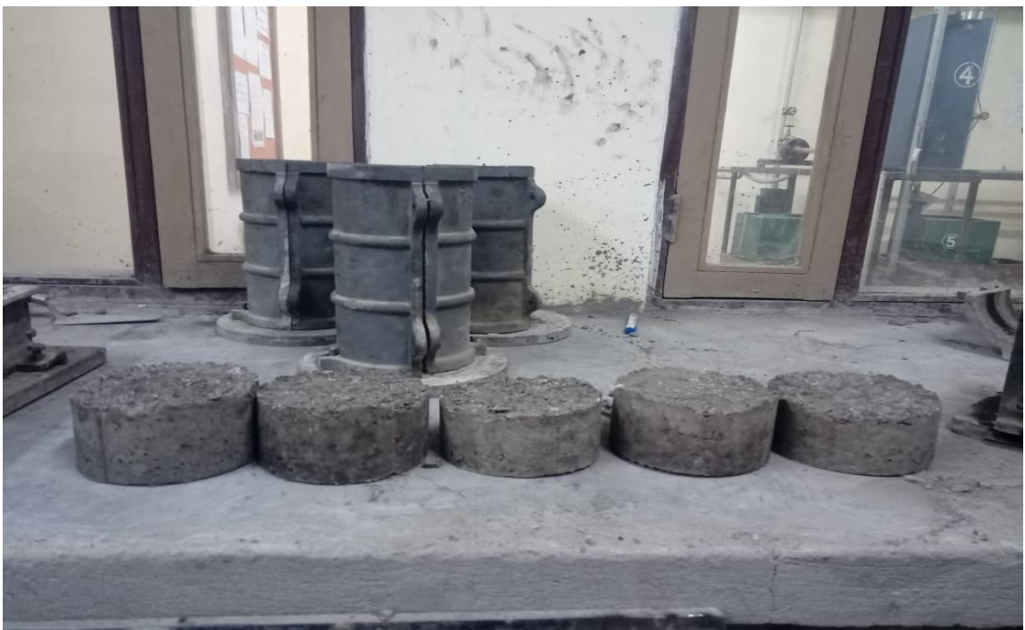
Figure 3.9 Standard concrete specimens for drop weight impact test
