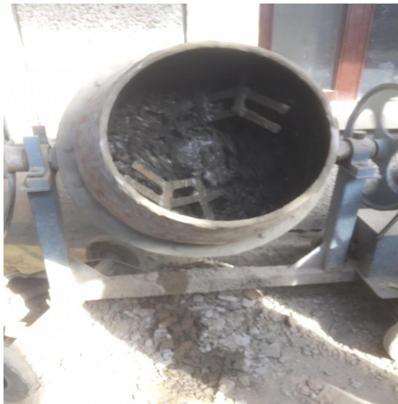
Figure 3.3 Concrete mixer used for preparing the concrete mix
