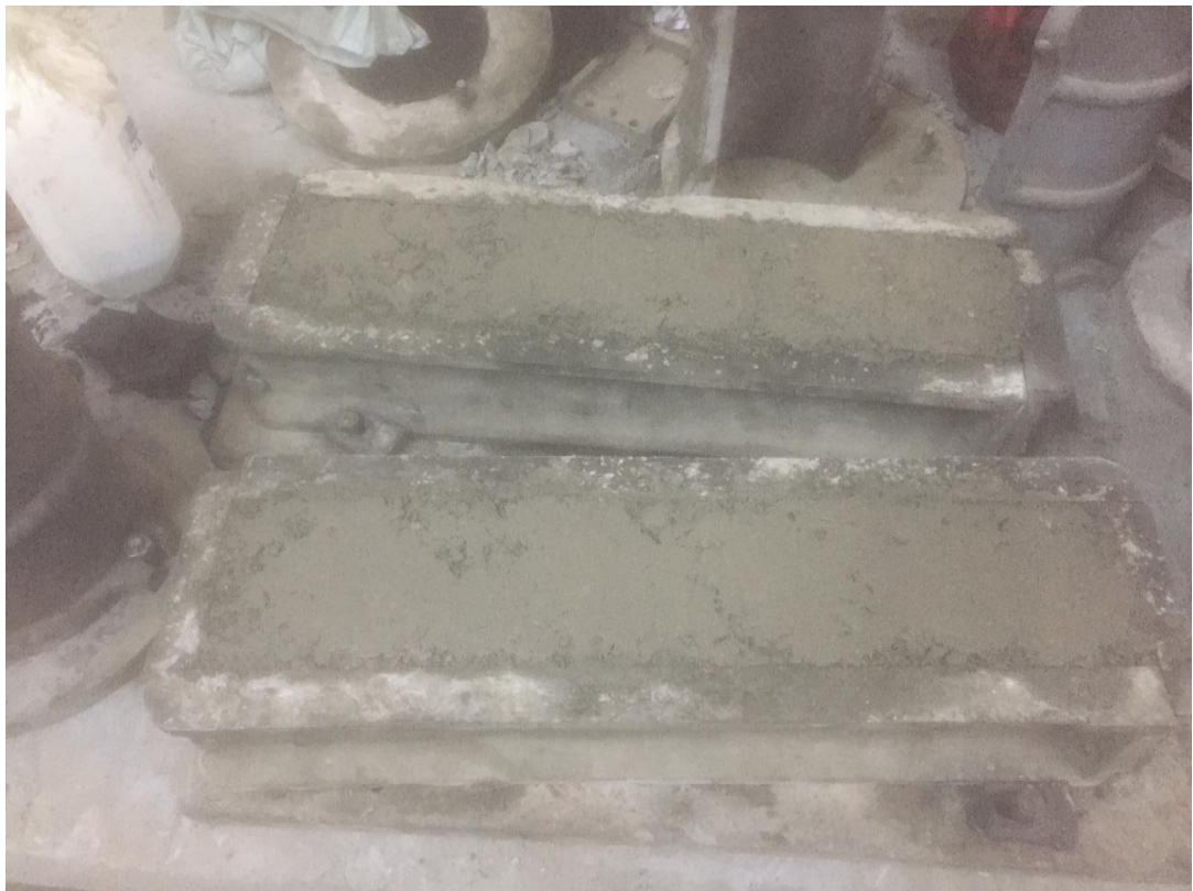
Figure 3.5 Casted concrete beams specimen for flexural testing
