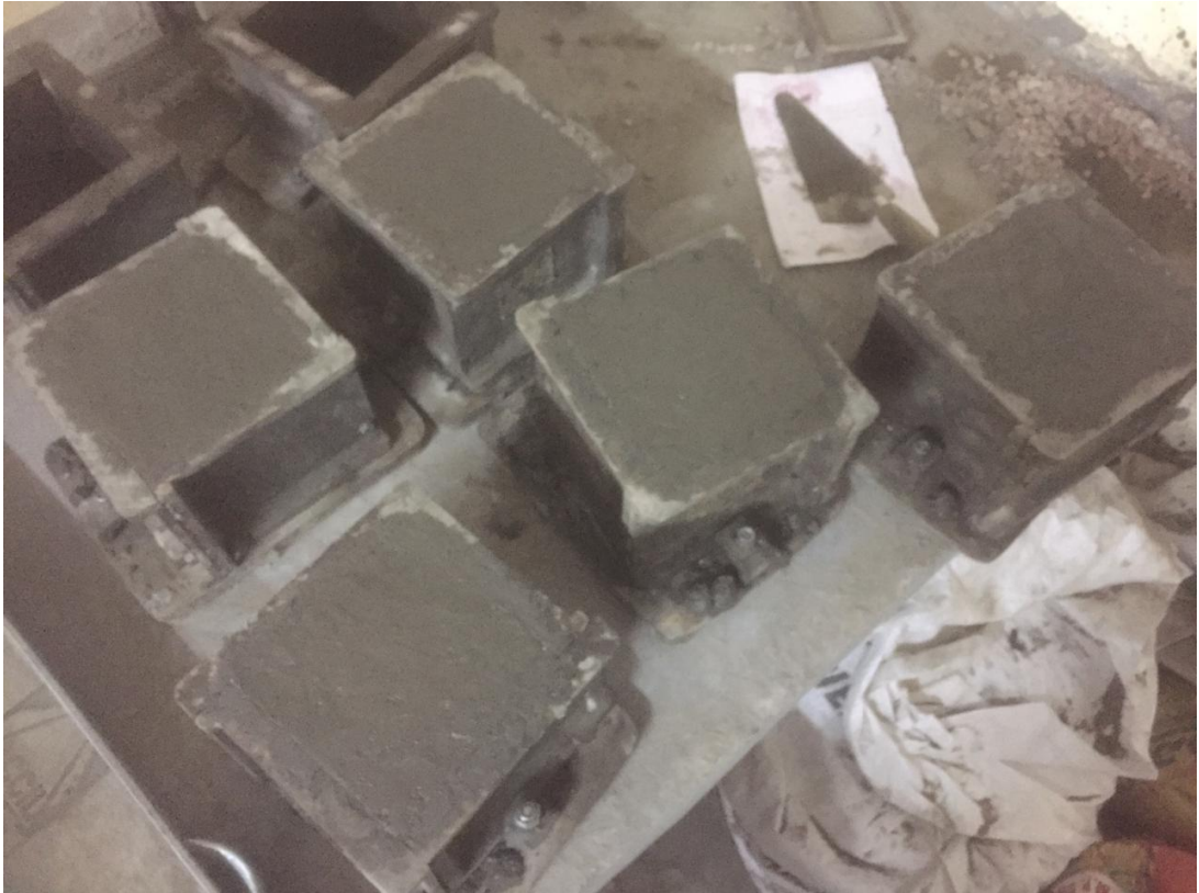
Figure 3.6 Fresh concrete cubes for compression test
