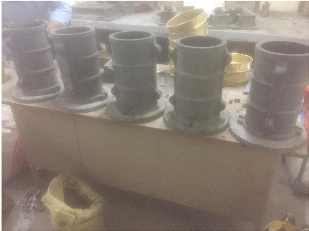
Figure 3.4 Cylindrical moulds used in casting of standard concrete specimen for impact test
