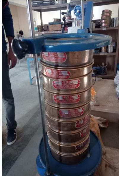
Figure 3.1 Standard test apparatus for sieve analysis of fine aggregates
