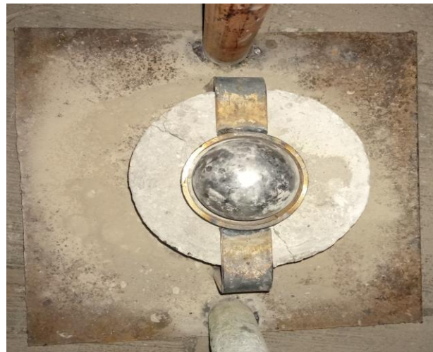
Figure 3.14 Drop weight test apparatus base plate with steel ball and casted cylinder
