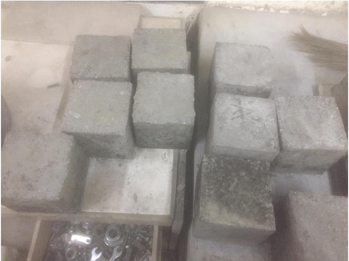
Figure 3.8 Cubes of 150 mm diameter containing 0.5 % Steel fibre
