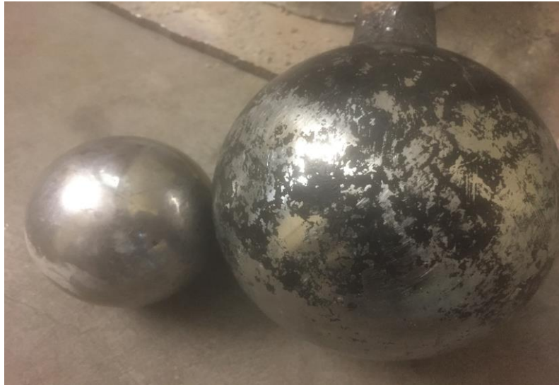
Figure 3.15 steel ball(1.054kg ), cast iron ball(4.500 kg) according to ACI 544
