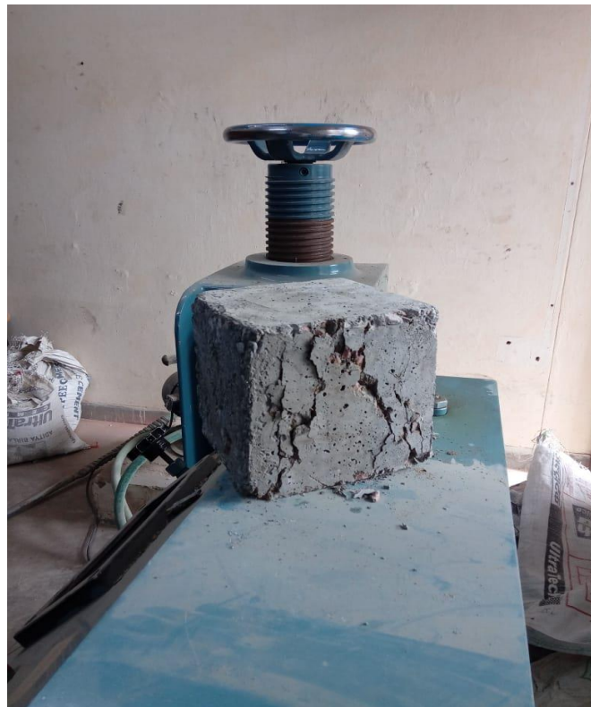
Figure 4.3 Failure of concrete cube under compressive loading.
