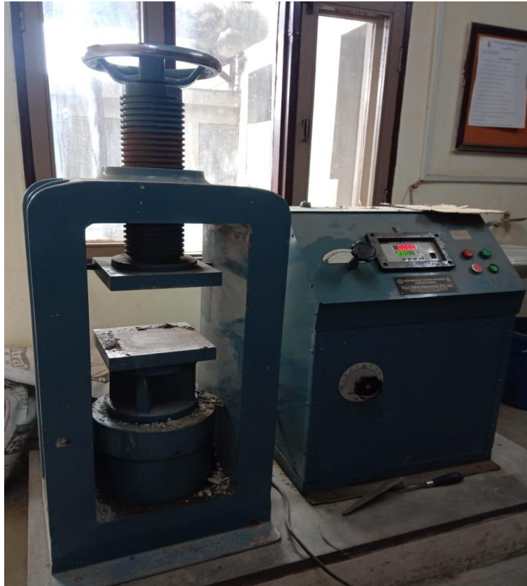
Figure 3.11 Load control Compression Testing Machine of capacity 2000 kN for compression testing
