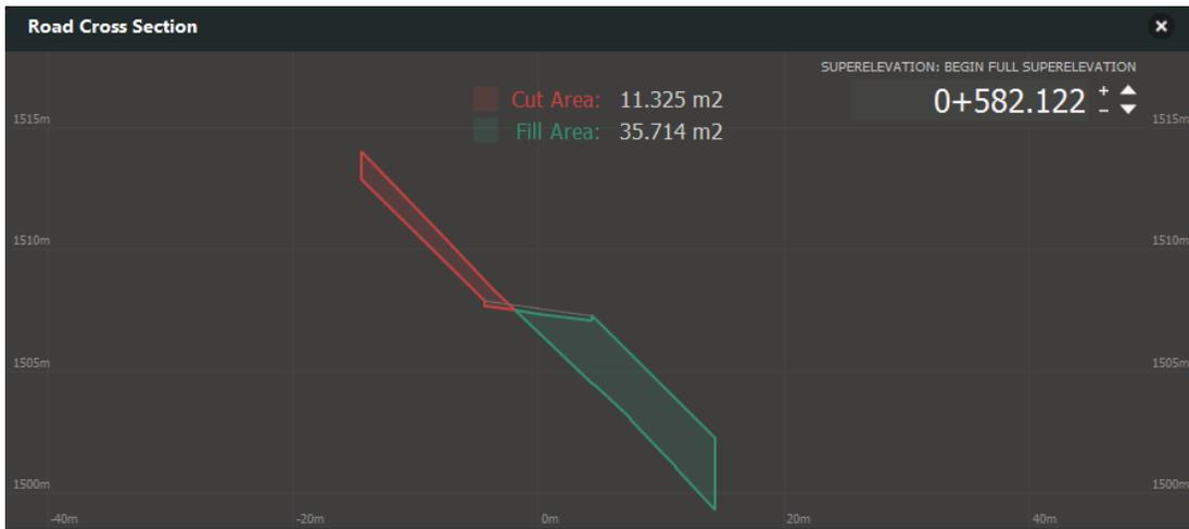
Figure 2.21C Cut-fill area at station 0+582.122
