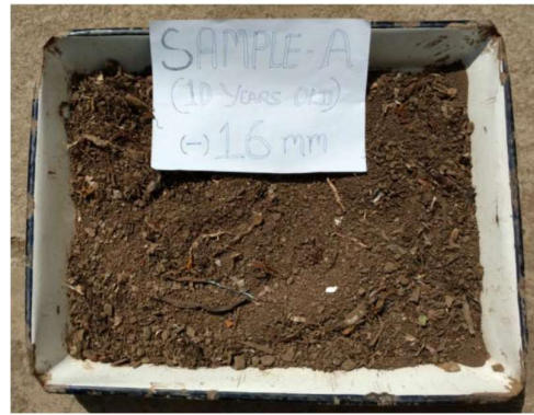
Figure 1.5(b) Sieved Sample (16mm)
