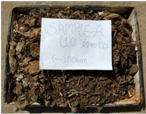
Figure 1.5(a) Sieved sample (80mm)
