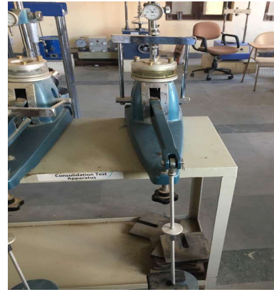
Figure 3.7(b) Oedometer setup
