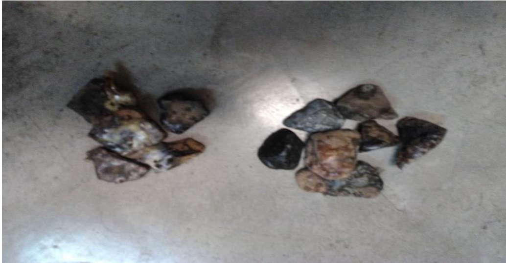
Figure 3.3 - Plastic Waste Coated Aggregates in JUIT Highway Lab
