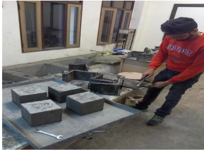
Fig 4.7: Demoulding of cubes
