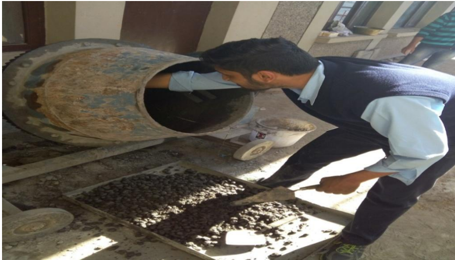
Fig 4.3: Concrete Mixing using laboratory mixer
