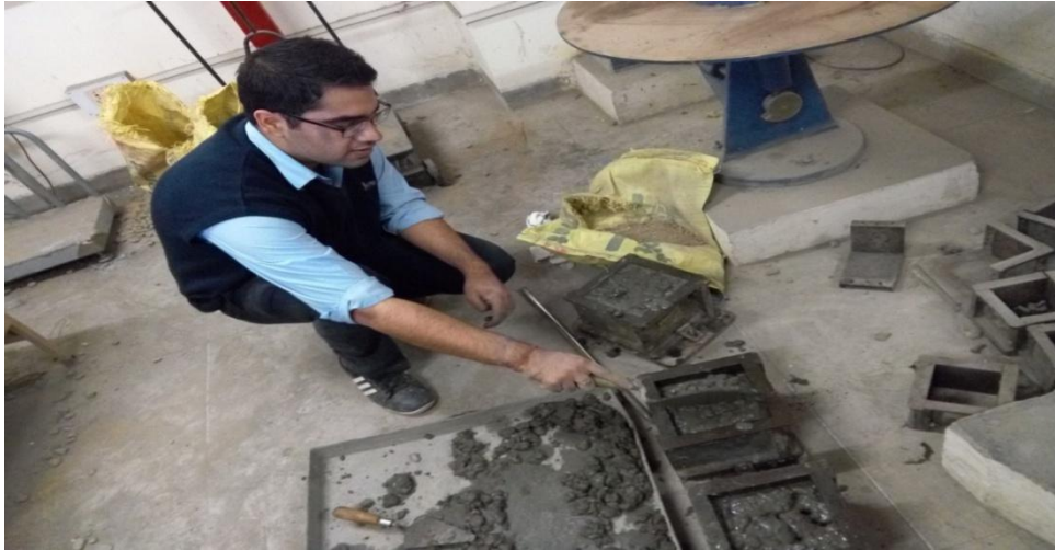
Fig 4.6: Casting of cubes by student Kshitij Tandon
