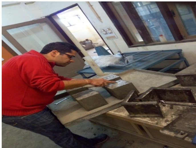
Fig 4.8: Marking cubes for identification
