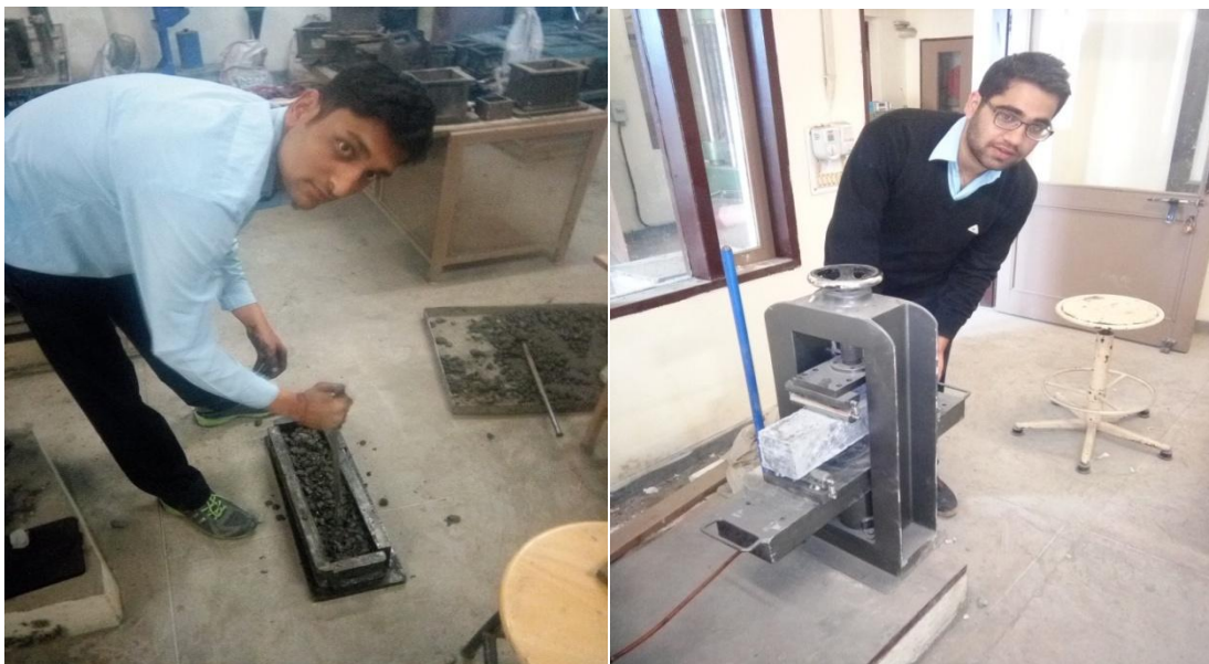
Fig 4.15: Casting of Beam and Flexural Strength Test
