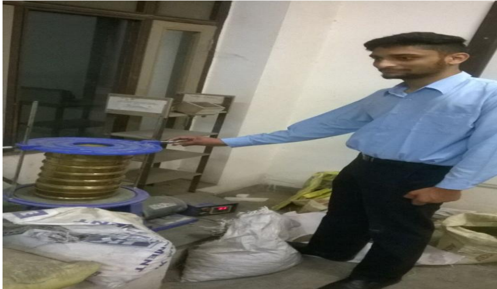
Fig 4.2: Sieve Analysis performed by student Mohit Thakur
