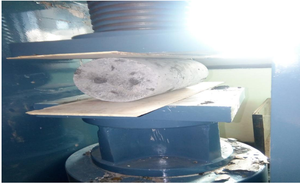
Fig 4.12: Split Tensile Strength Test.
