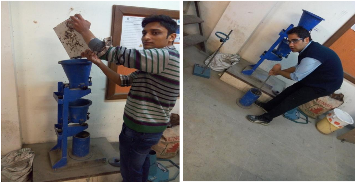
Fig 4.5: Students performing Compaction Factor Test.
