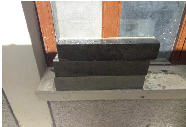
Fig 4.14: Beams casted for Flexural Strength Test
