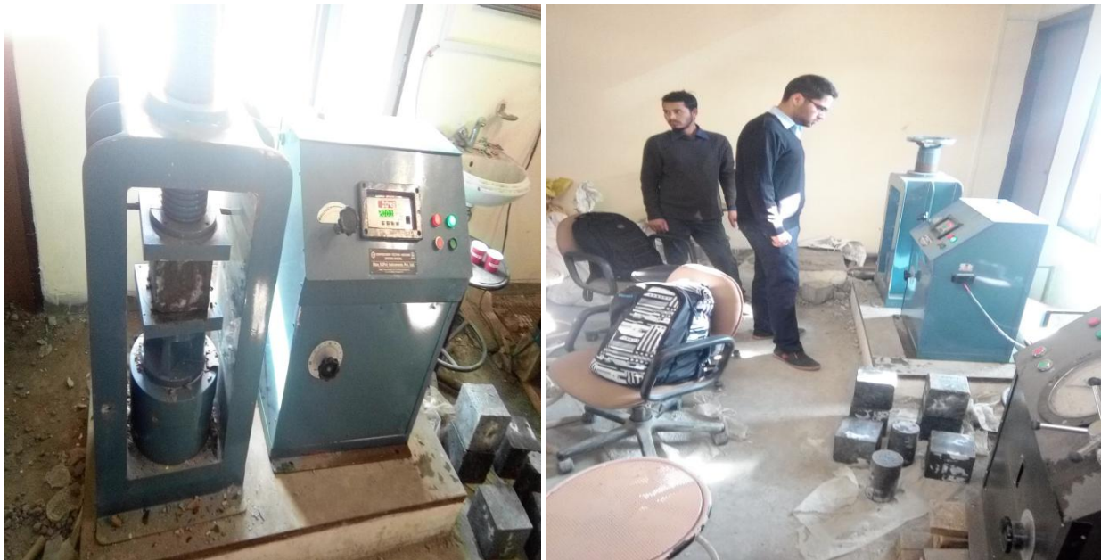
Fig 4.11: Compression Strength Testing
