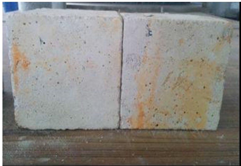
Fig 4.18: Chloride Attack Test (Hydrochloric Acid)
