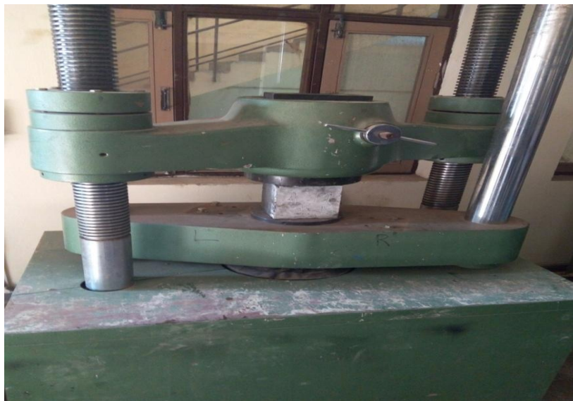
Fig 4.10: Compressive Strength Test on Universal Testing Machine.
