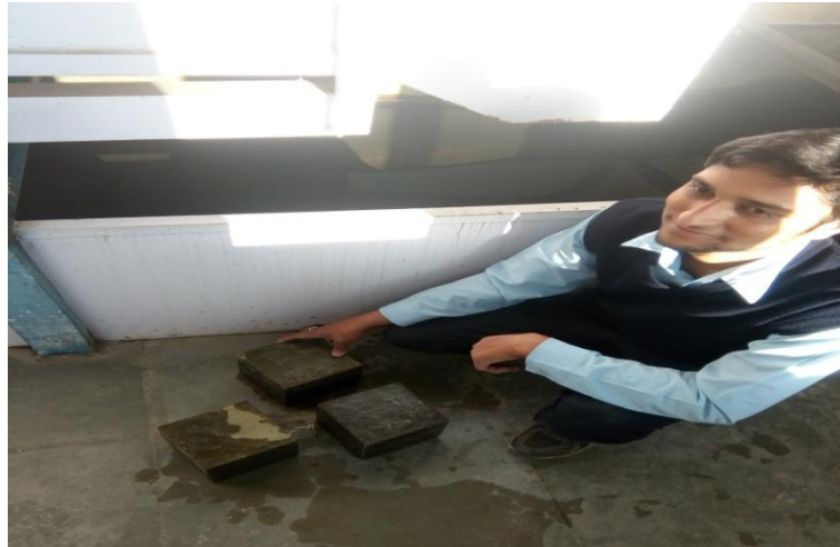
Fig 4.9: Student showing cubes taken out of curing tank
