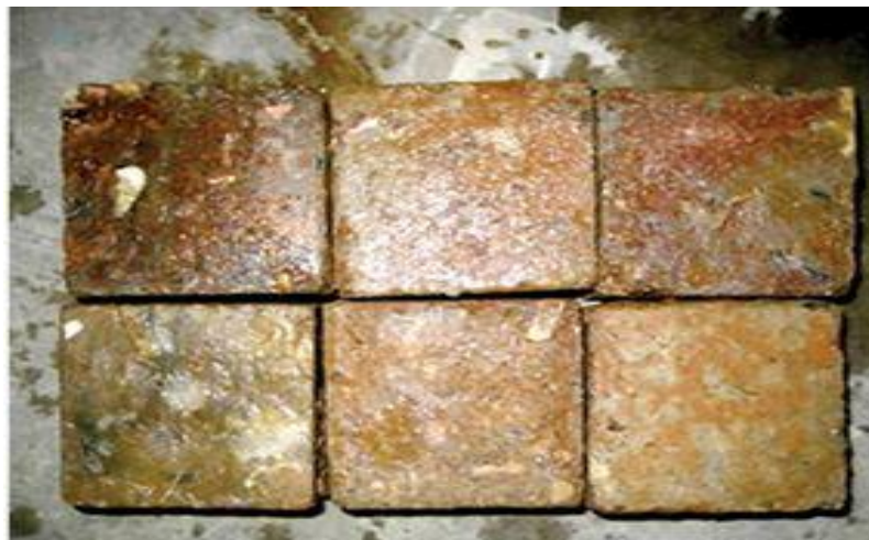
Fig 4.17: Acid Attack Test (Sulphuric acid)
