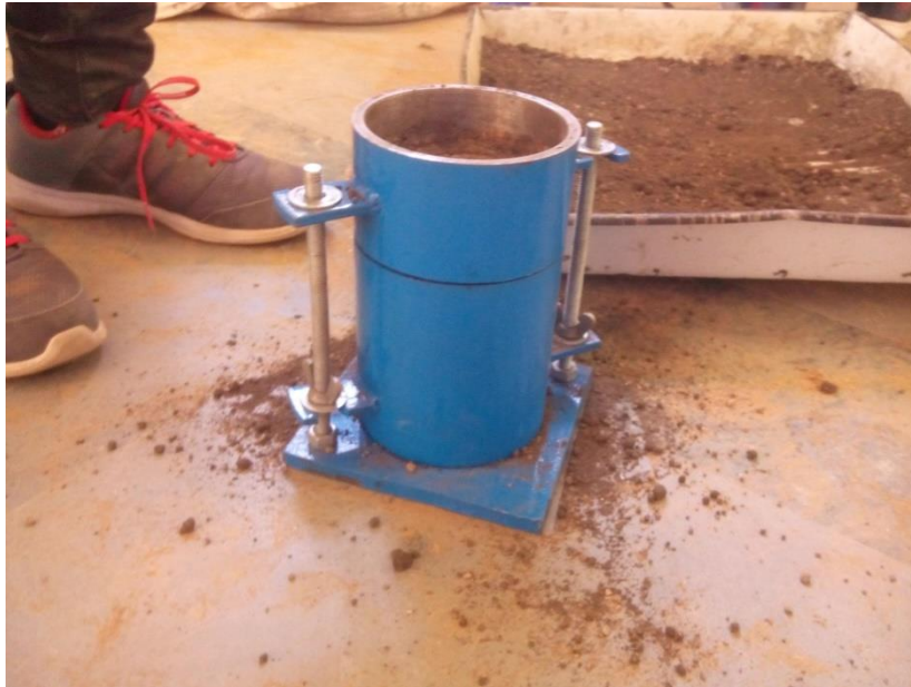
FIGURE 3.6: Light Weight Compaction Test
