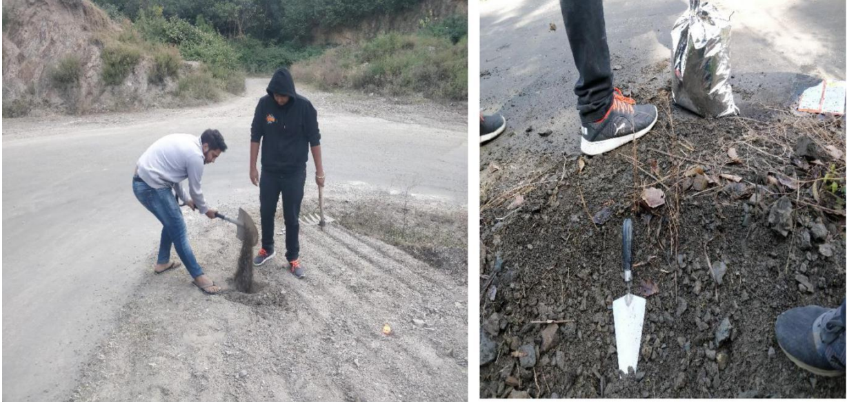
Fig. 3.3 and 3.4 Collection of Soil Samples for CBR test
