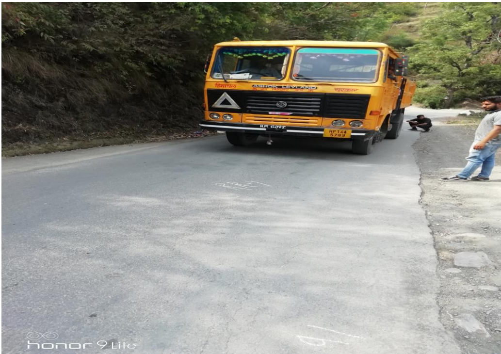
Fig 4.11 Marked distances before movement of truck at RR4
