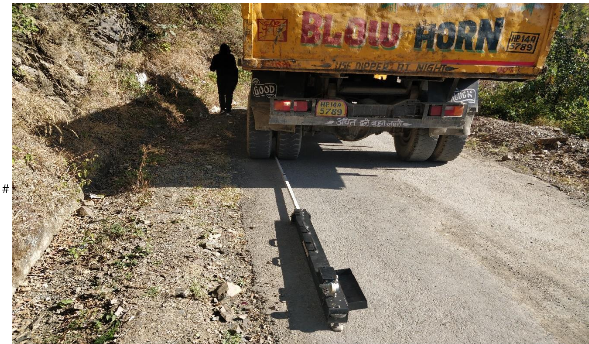
Fig. 4.3 Benkelman Beam in middle of rear axle rear Axle of truck
