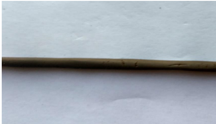
Fig 3.7: Soil thread crumbles at 3 mm diameter
