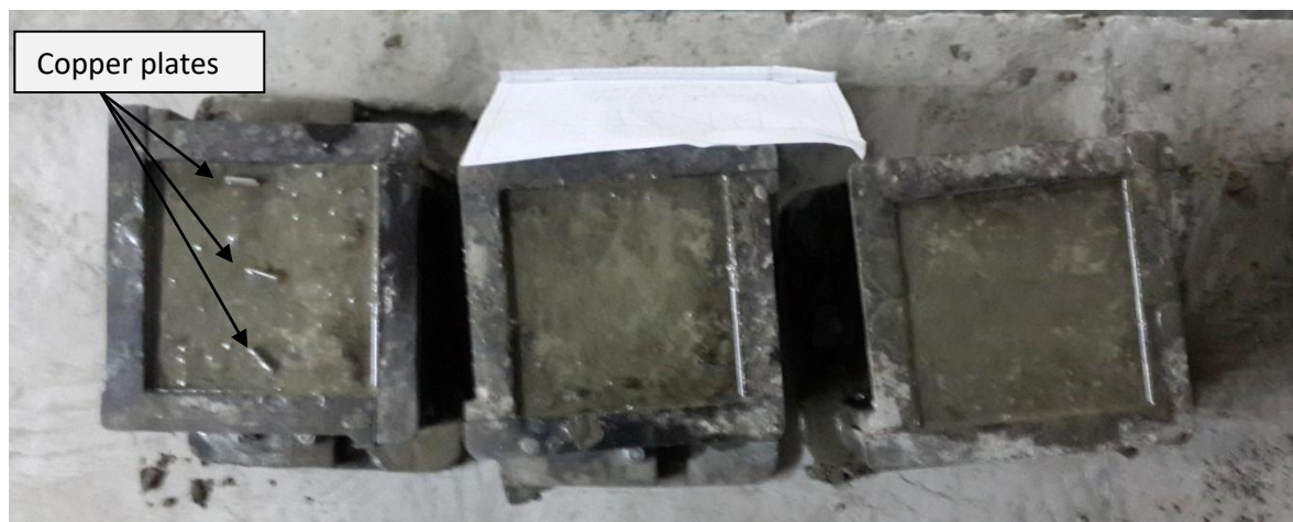
Figure 3.7 Concrete cube specimens with cracks induced (left) and without cracks (middle and right)
