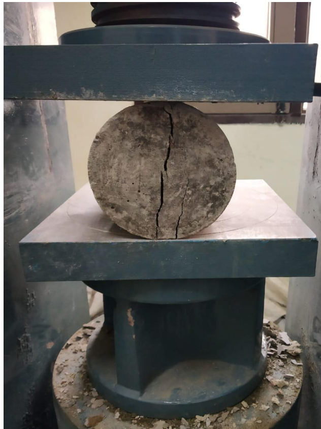
Figure 3.5 Failure of concrete cylinder under CTM
