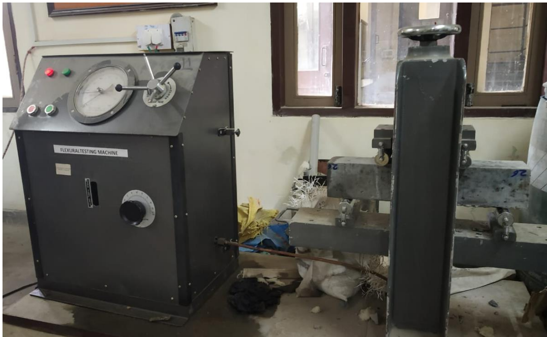
Figure 3.6 Flexural strength test setup under flexural testing machine
