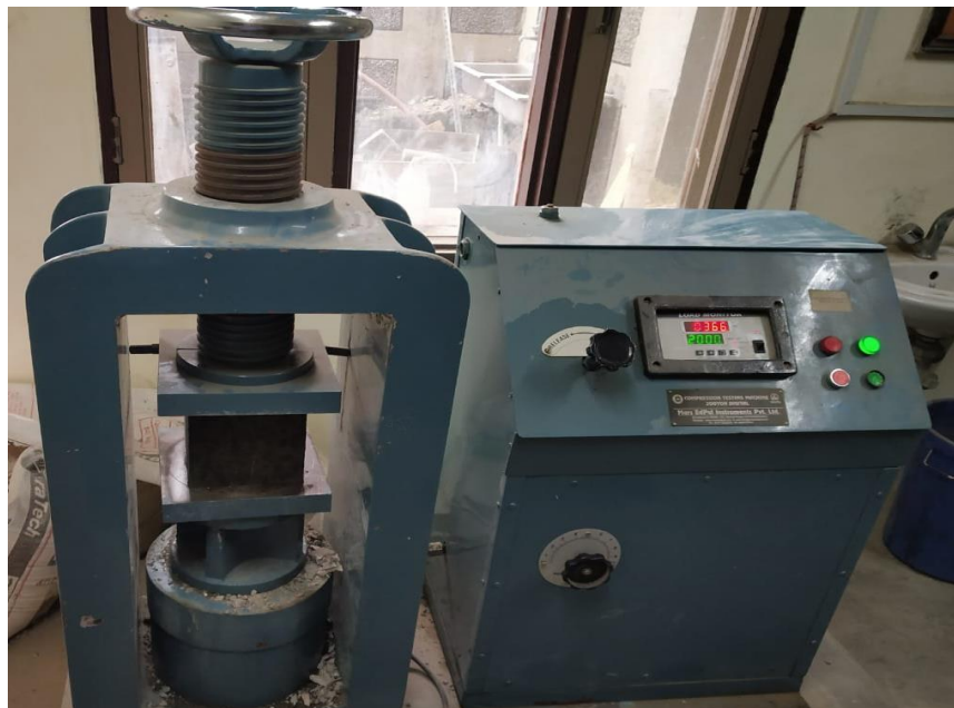
Figure 3.4 Compressive strength test setup under CTM
