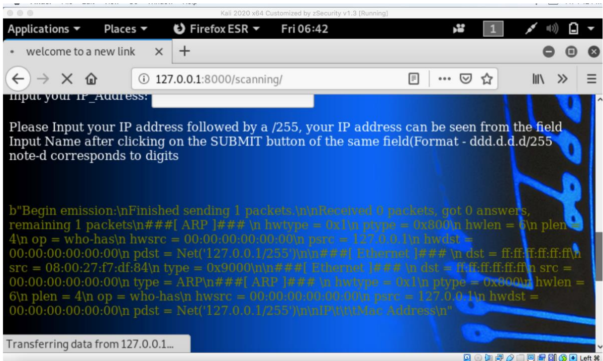
Figure 25:- Retrieval of IP address of connected devices
