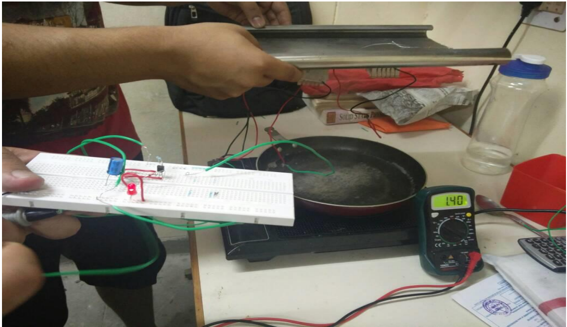
Fig 4.11: Final circuit (including both thermopile and booster circuit)
