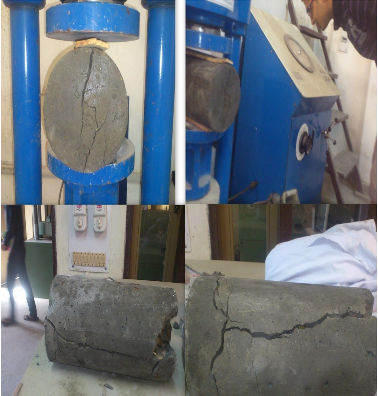
Figure 4. Split tensile test after 7 days curing
