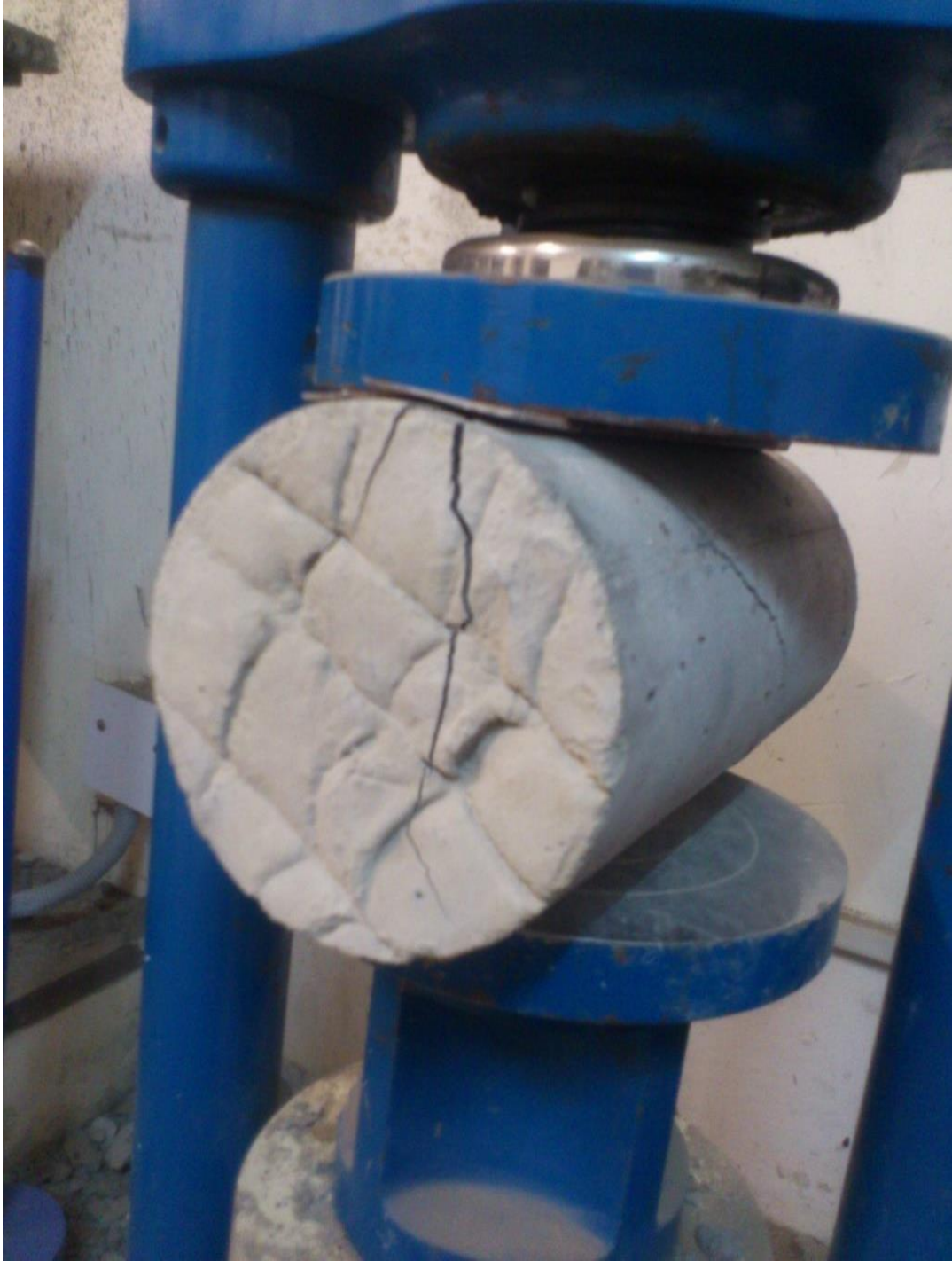
Figure 6. Split tensile test after 28 days curing
