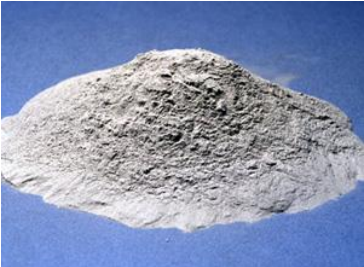
Figure 2.5 Fly ash, powder resembling cement, has been used in concrete since the 1930s
