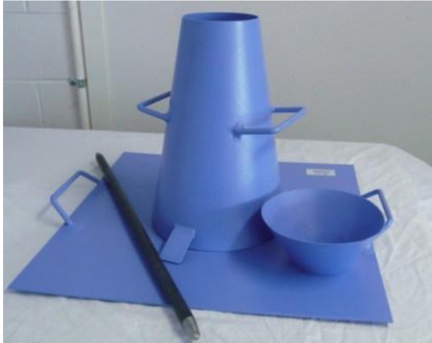
Fig 5.4 Slump Cone Test Apparatus
