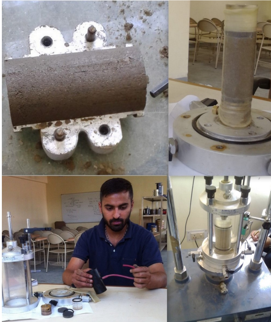
Figure 17 Extraction of sample and setting the sample to perform test
