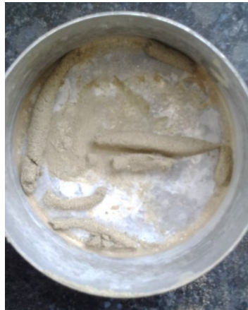
Figure 14 Soil could not be rolled into threads
