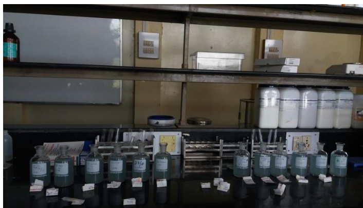
Fig 3.2 Sample bottles with 12 different sample for BOD studie
