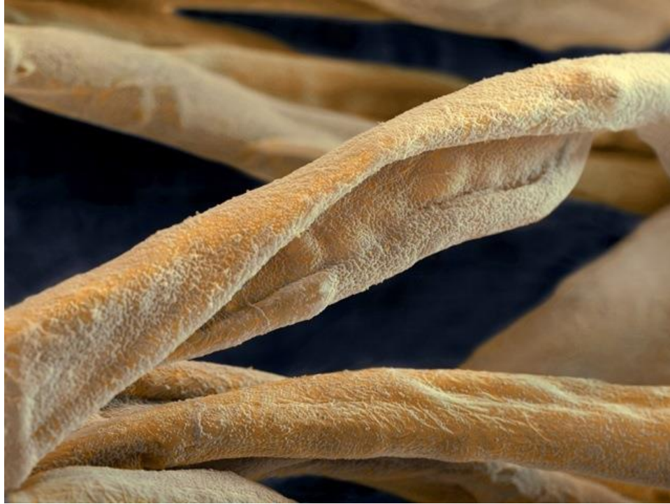
Figure 6. Nanoparticles create a structure on the surface of these textile fibres that mimics the leaves of a lotus plant, making them water and dirt repellent. Sharon et al. (2015)
