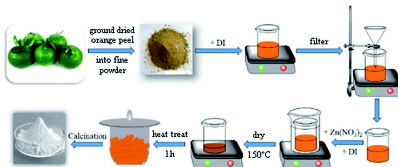
Figure 11 Schematic diagram of the green synthesis of ZnO nanoparticles. T. U. Doan et al. (2020)
