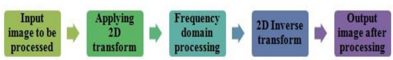
Fig.1.8: The main steps in transform domain fusion technique.
