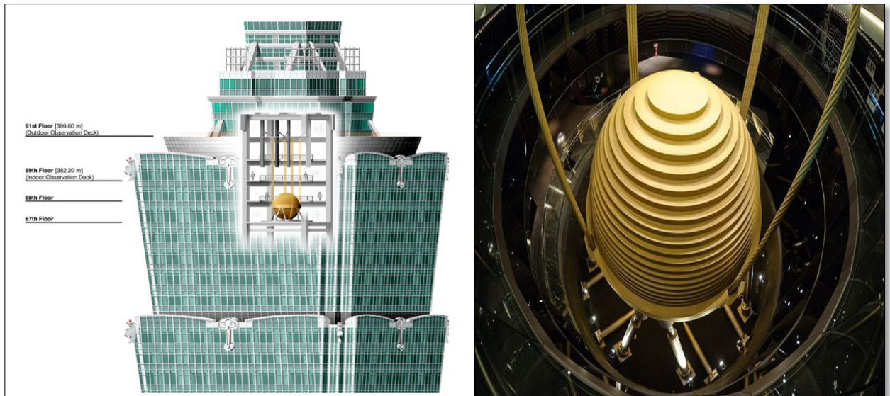
Figure 18 Enormous pendulum (TMD) helps keep Taiwan's tallest building, Taipei from swaying
