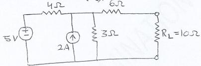
Q3. Determine node voltages of the circuit given below using Nodal analysis:
