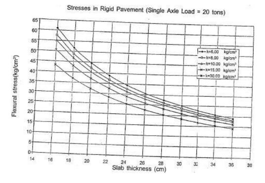
Stress in rigid pavement for 20 ton single axle load
