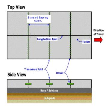
Fig 3.10: Different views of tie bar and dowel bar
