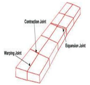
Fig 3.8: Showing different types of joints
