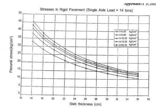
Stress in rigid pavement for 14 ton single axle load
