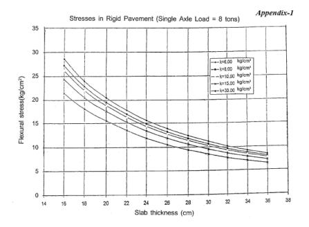
Stress in rigid pavement for 8 ton single axle load
