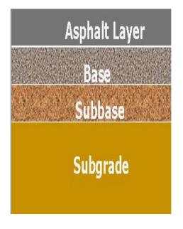
FIG 1.1(A) Flexible Pavement
