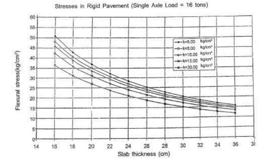
Stress in rigid pavement for 16 ton single axle load
