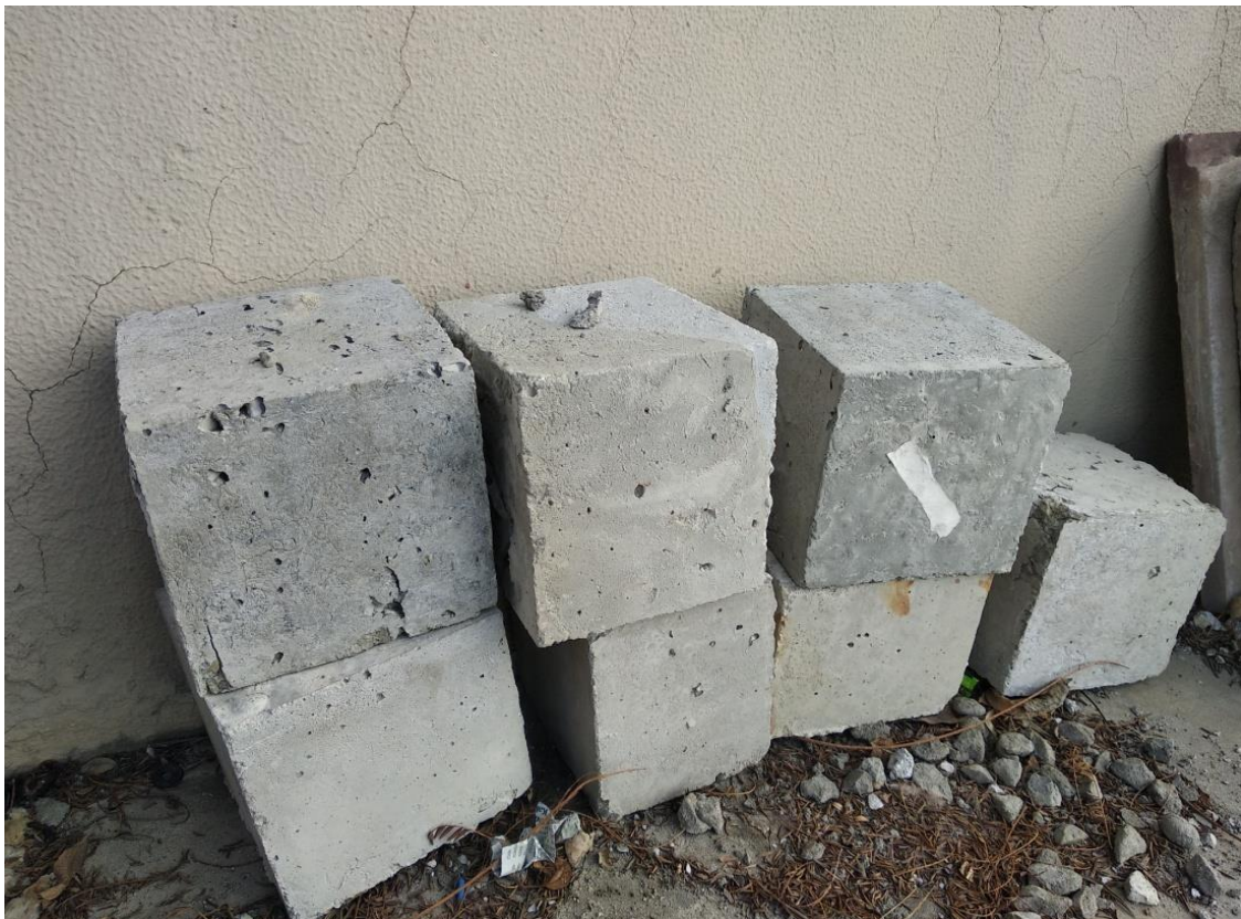
Fig. 3.13 Curing of cubes in sunlight
