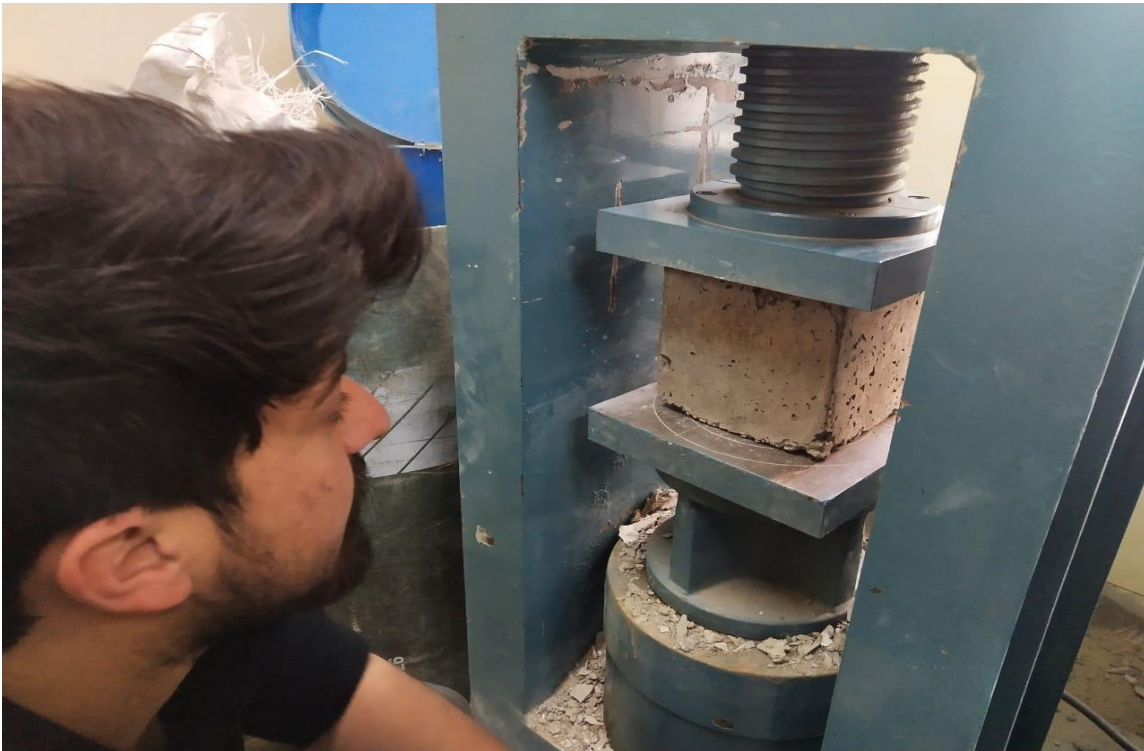
Fig. 3.15 Testing of cubes under CTM
