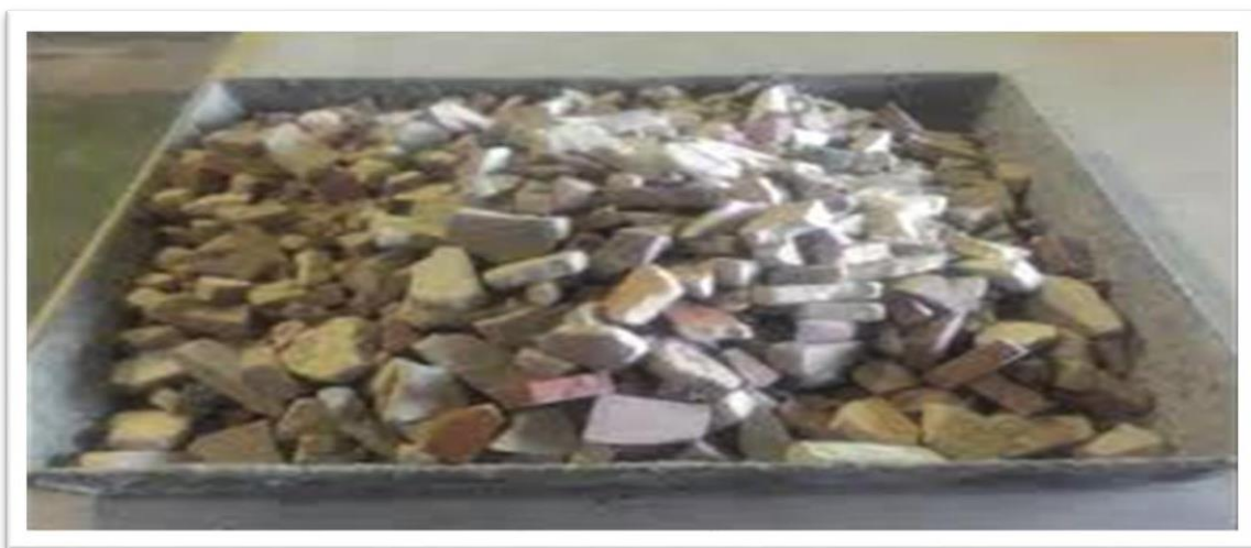
Fig.3.6 Waste crushed tiles used as replacement of Coarse Aggregate
