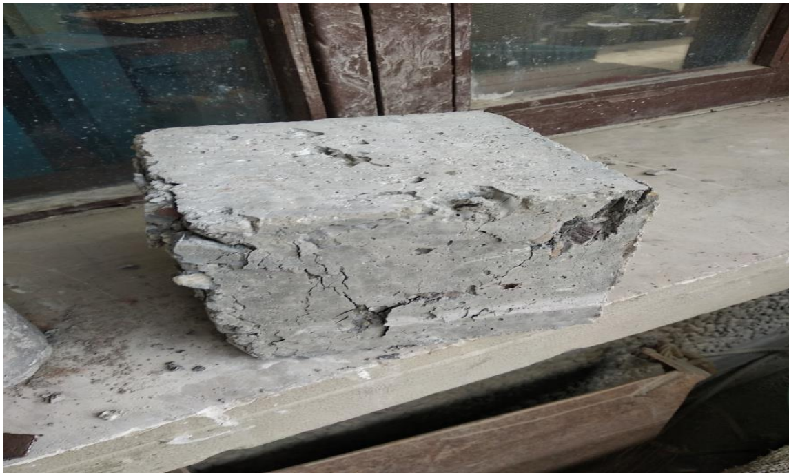
Fig. 3.17 Crumb rubber cube after cracks under CTM
