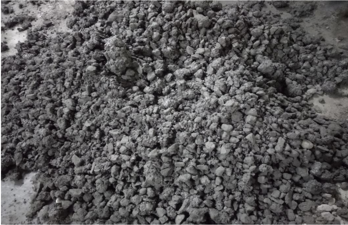
Fig. 3.12 Crumb rubber is mixed in concrete
