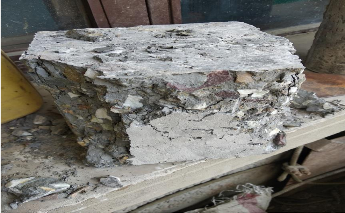
Fig. 3.16 Waste tiles cube after cracks under CTM
