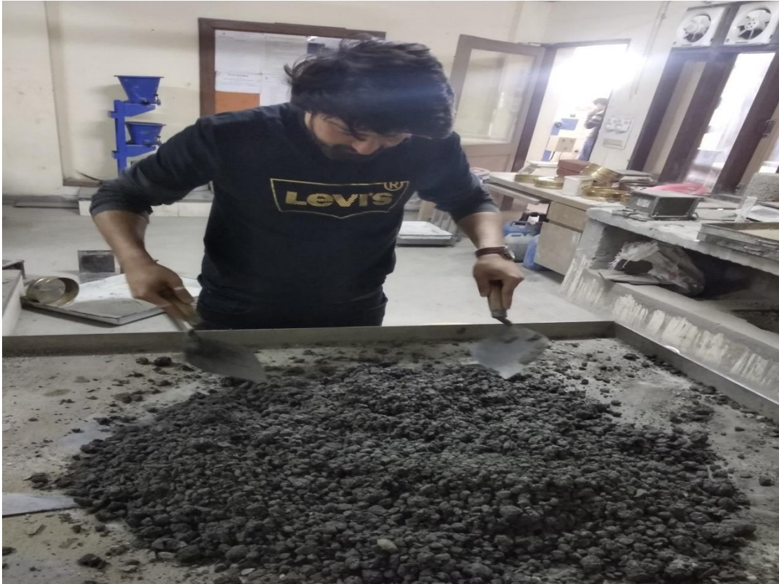
Fig. 3.10 Bagasse is added in concrete mix
