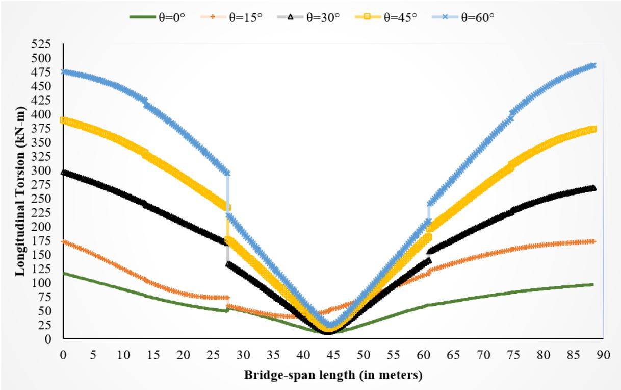
a) Longitudinal Torsion for bridge models having Curvature Angle ( $\beta$ ) of 30° with different Skew Angles under Longitudinal Excitations
