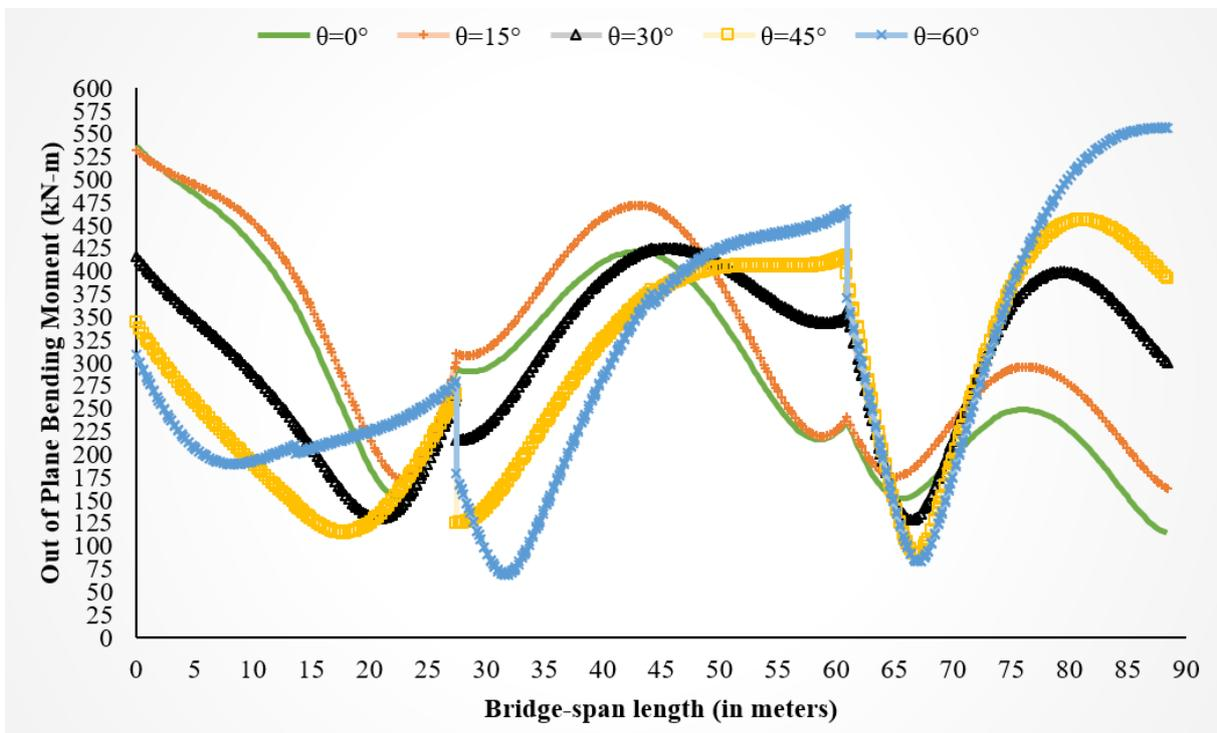
c) Out-of-Plane Bending Moment for bridge models having Curvature Angle ( $\beta$ ) of  $90^\circ$  with different Skew Angles under Longitudinal Excitations
