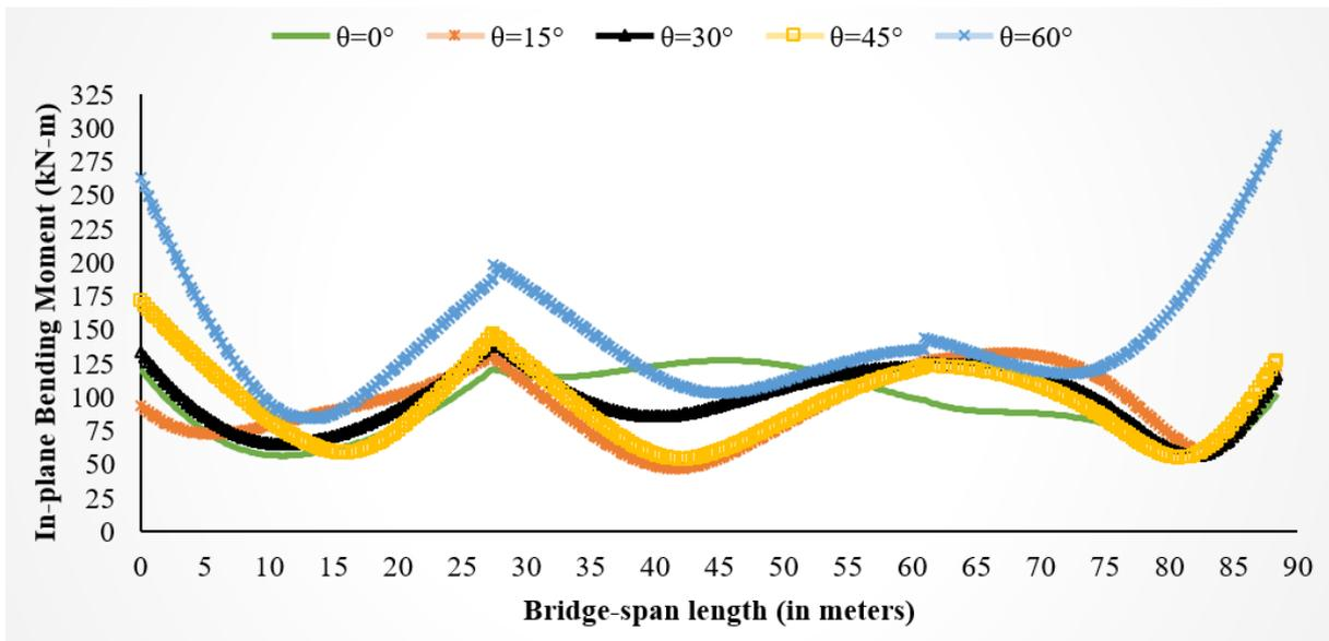
c) In-plane Bending Moment for bridge models having Curvature Angle ( $\beta$ ) of  $90^\circ$  with different Skew Angles under Vertical Excitations
