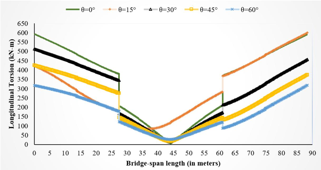
a) Longitudinal Torsion for bridge models having Curvature Angle ( $\beta$ ) of  $30^\circ$  with different Skew Angles under Transverse Excitations
