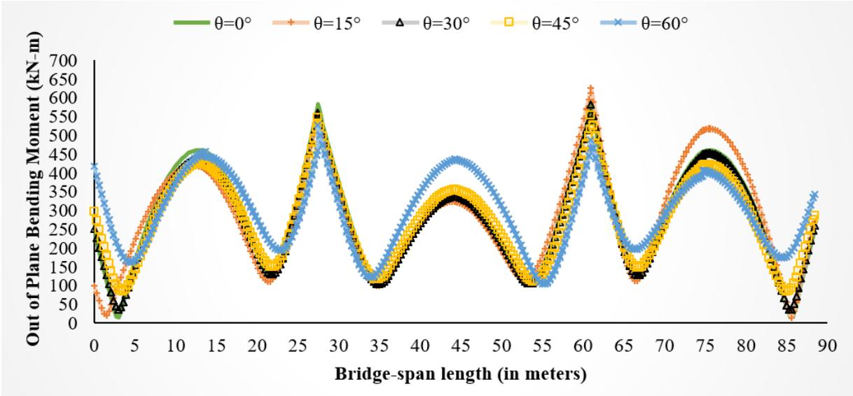
Figure 5.4 Out-of-Plane Bending Moment for bridge models having Curvature Angle ( $\beta$ ) of  $0^\circ$  with different Skew Angles under Vertical Excitations
