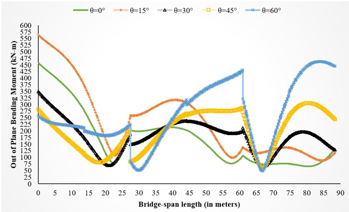
b) Out-of-Plane Bending Moment for bridge models having Curvature Angle ( $\beta$ ) of  $60^\circ$  with different Skew Angles under Longitudinal Excitations
