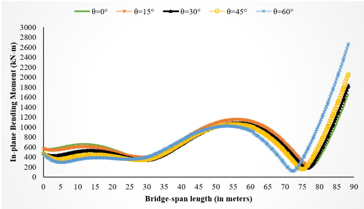
b) In-plane Bending Moment for bridge models having Curvature Angle ( $\beta$ ) of  $60^\circ$  with different Skew Angles under Longitudinal Excitations
