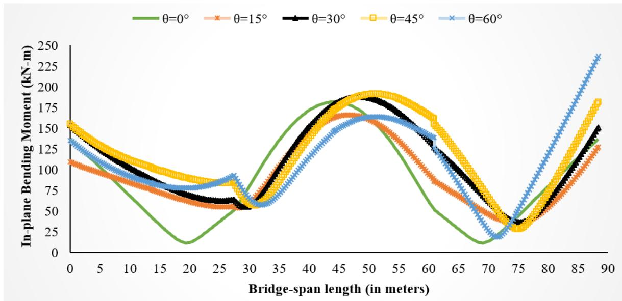
**Figure 5.7** In-plane Bending Moment for bridge models having Curvature Angle ( $\beta$ ) of  $0^\circ$  with different Skew Angles under Vertical Excitations
