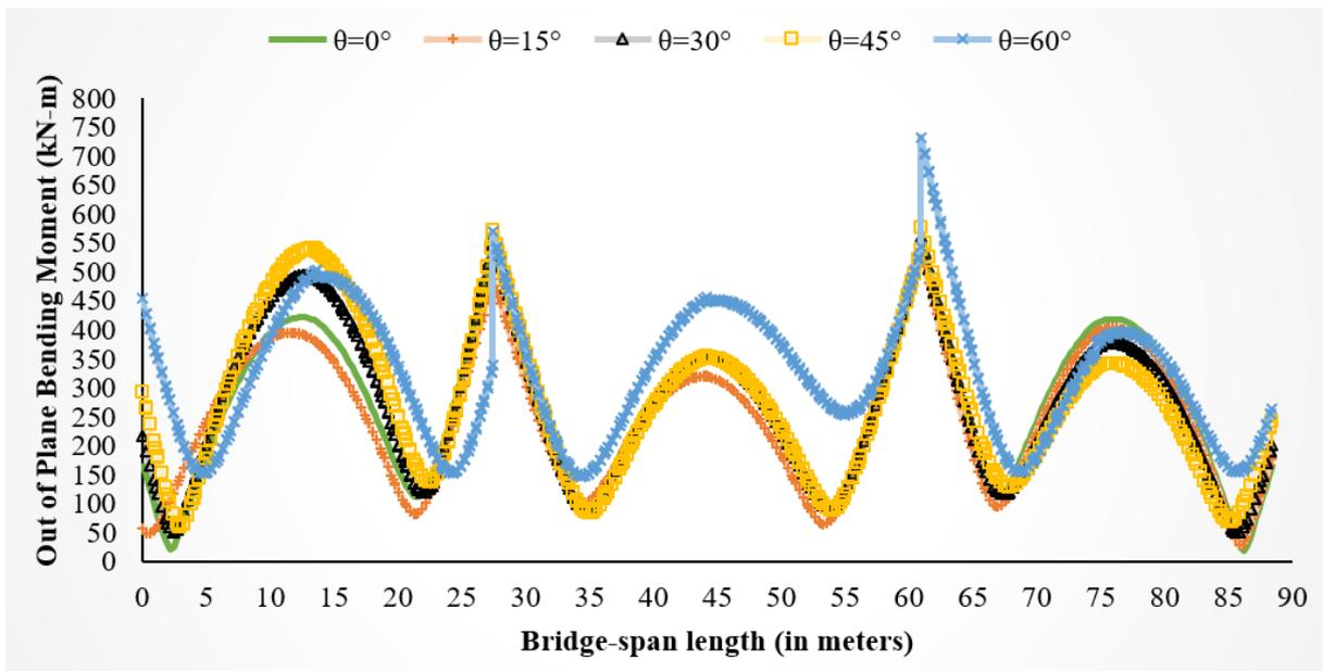
c) Out-of-Plane Bending Moment for bridge models having Curvature Angle ( $\beta$ ) of  $90^\circ$  with different Skew Angles under Vertical Excitations
