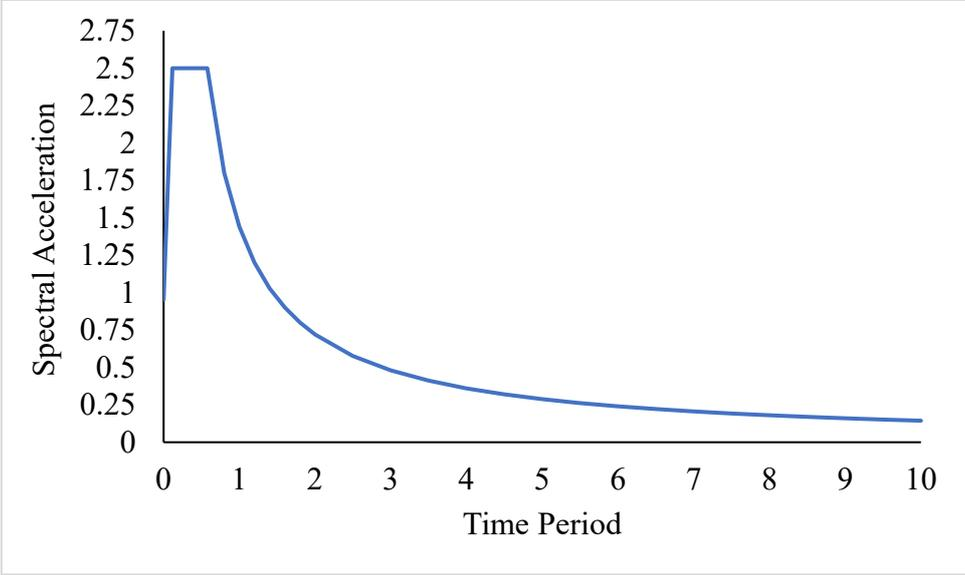
Figure 5.1 Response Spectrum AASHTO 2007 Function Graph
