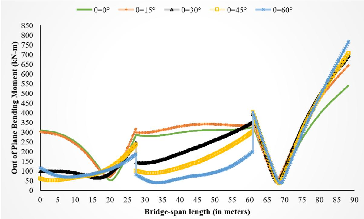
b) Out-of-Plane Bending Moment for bridge models having Curvature Angle ( $\beta$ ) of  $60^\circ$  with different Skew Angles under Transverse Excitations
