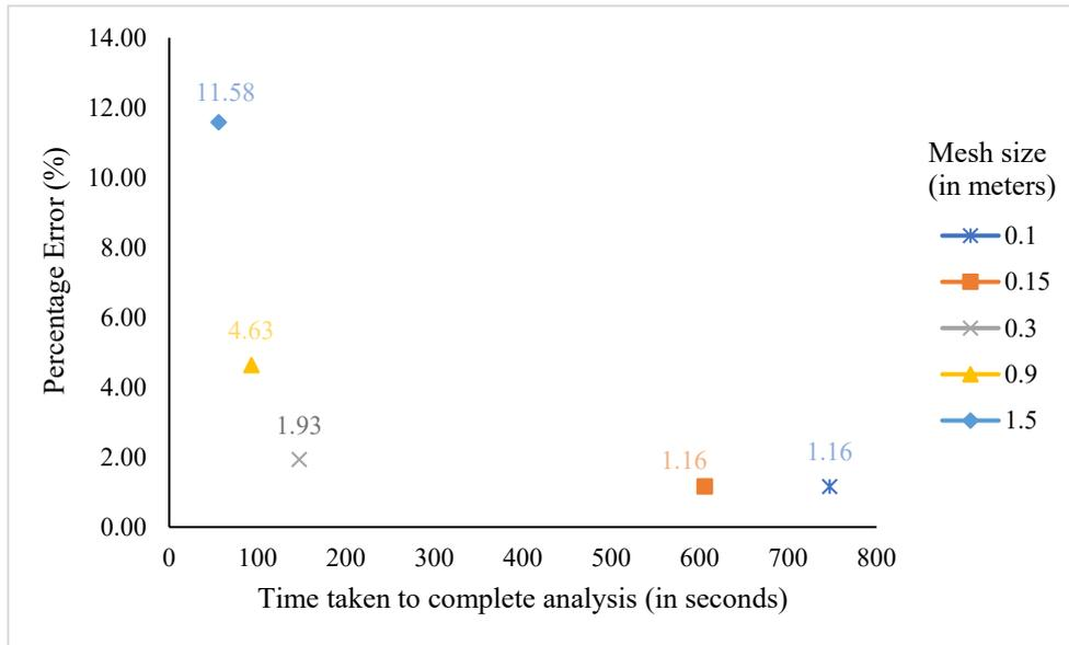
**Figure 3.7** Percentage Error versus Analysis Time graph for different mesh sizes
