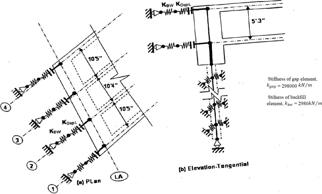
Figure 3.13 Modelling details of gap element and backfill element [94]
