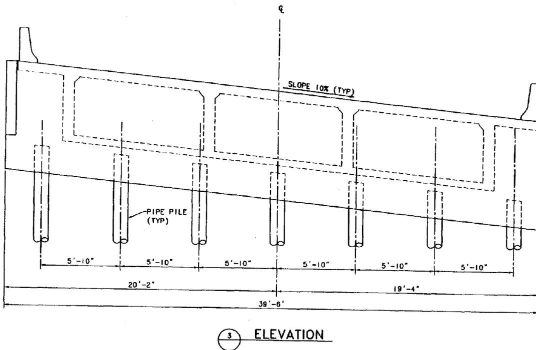
Figure 3.4 Abutment details of Benchmark Bridge [93]
