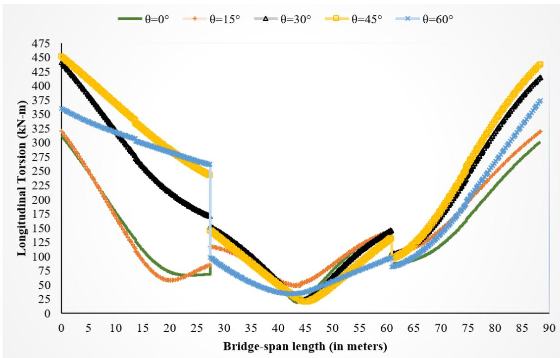
c) Longitudinal Torsion for bridge models having Curvature Angle ( $\beta$ ) of  $90^\circ$  with different Skew Angles under Longitudinal Excitations
