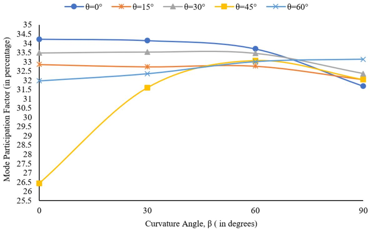
**Figure 4.8.** Mode Participation Factor of third Out of Plane Mode for various bridge configurations
