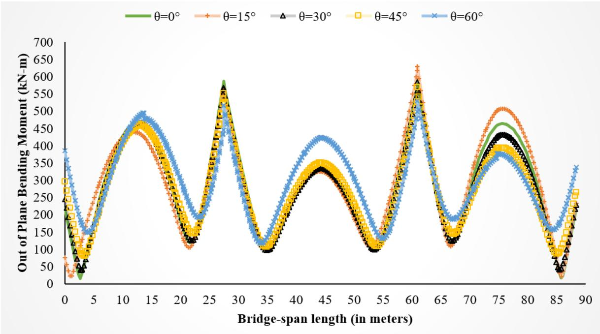
a) Out-of-Plane Bending Moment for bridge models having Curvature Angle ( $\beta$ ) of  $30^\circ$  with different Skew Angles under Vertical Excitations
