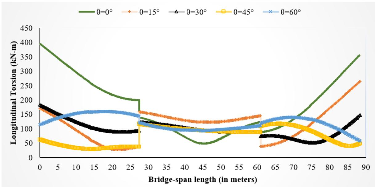
c) Longitudinal Torsion for bridge models having Curvature Angle ( $\beta$ ) of  $90^\circ$  with different Skew Angles under Transverse Excitations
