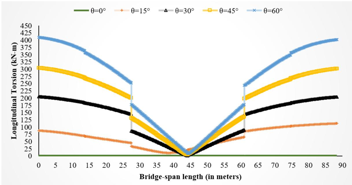
**Figure 5.8** Longitudinal Torsion for bridge models having Curvature Angle ( $\beta$ ) of  $0^\circ$  with different Skew Angles under Longitudinal Excitations
