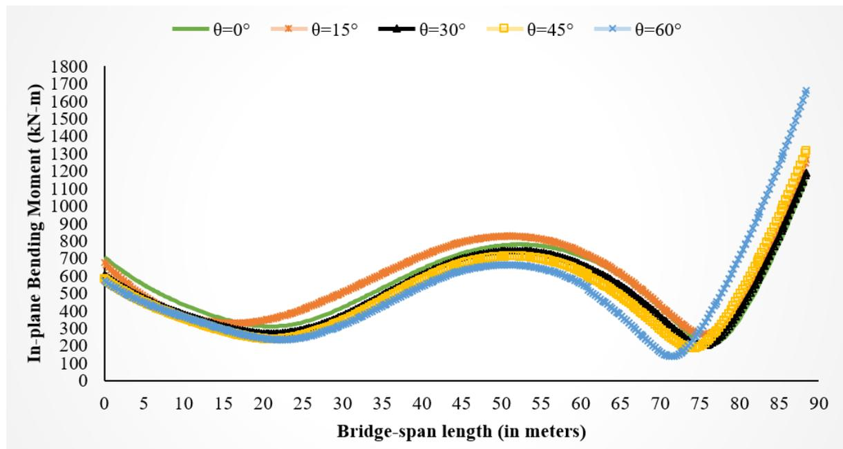
a) In-plane Bending Moment for bridge models having Curvature Angle ( $\beta$ ) of  $30^\circ$  with different Skew Angles under Longitudinal Excitations
