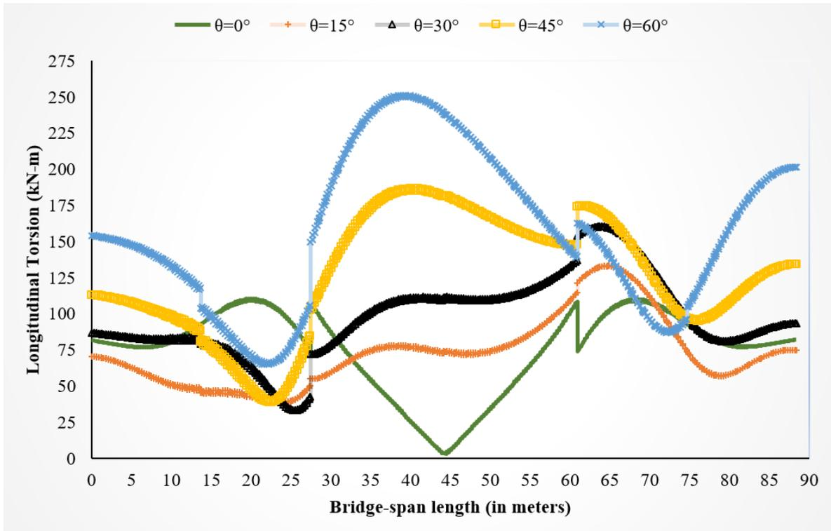
b) Longitudinal Torsion for bridge models having Curvature Angle ( $\beta$ ) of  $60^\circ$  with different Skew Angles under Vertical Excitations
