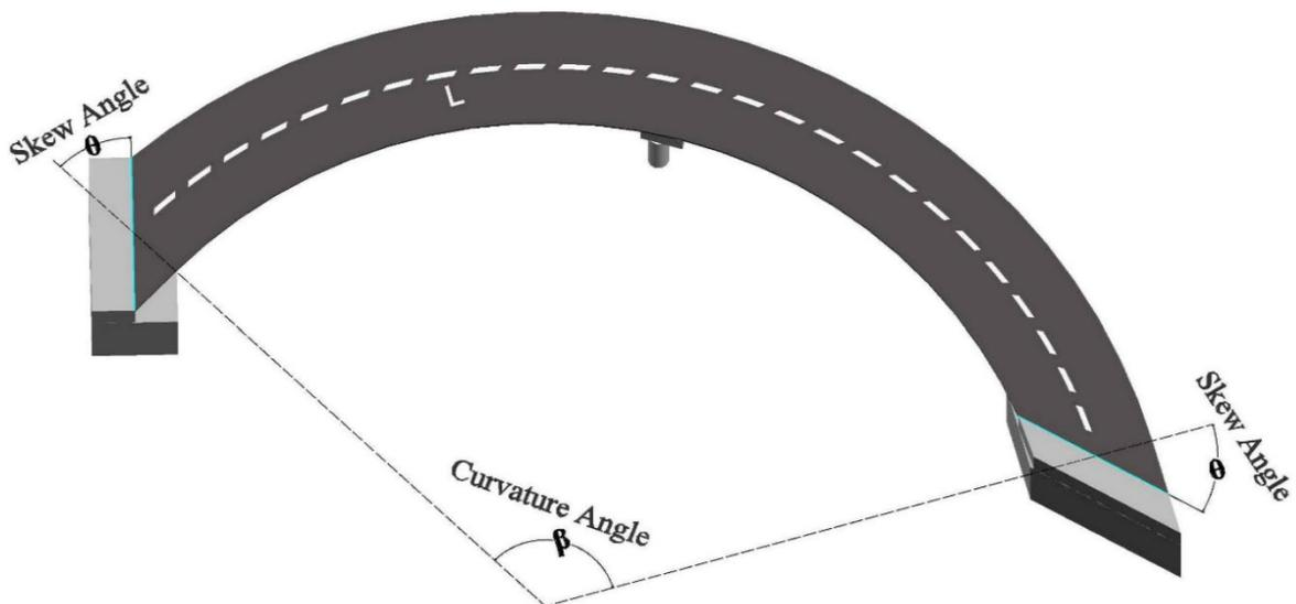
Figure 1.4 Skew-Curved Bridge Geometry
