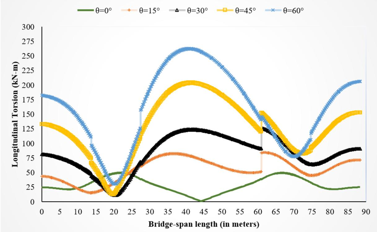
a) Longitudinal Torsion for bridge models having Curvature Angle ( $\beta$ ) of 30° with different Skew Angles under Vertical Excitations
