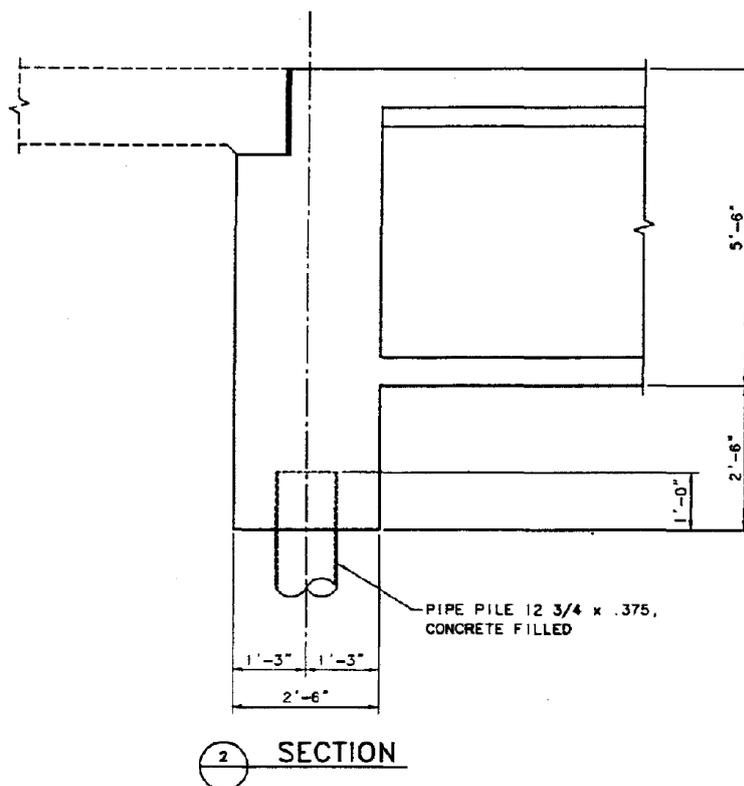
Figure 3.5 Details of pipe pile [93]
