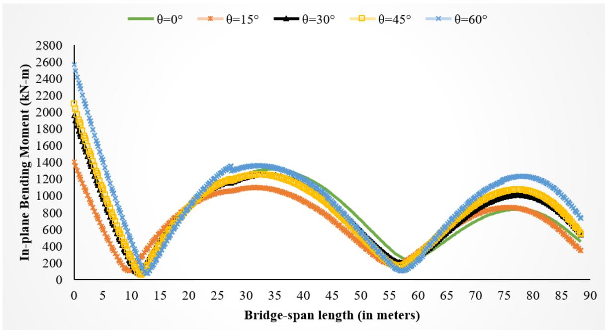
c) In-plane Bending Moment for bridge models having Curvature Angle ( $\beta$ ) of  $90^\circ$  with different Skew Angles under Transverse Excitations
