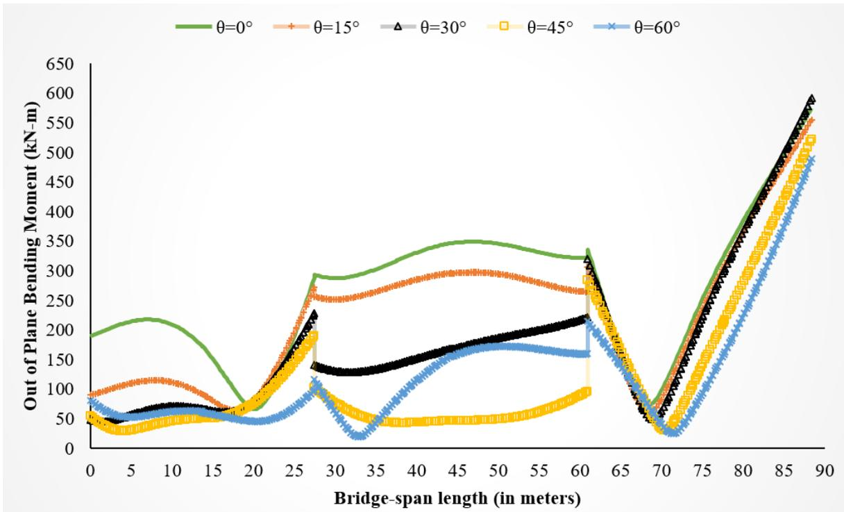
c) Out-of-Plane Bending Moment for bridge models having Curvature Angle ( $\beta$ ) of  $90^\circ$  with different Skew Angles under Transverse Excitations
