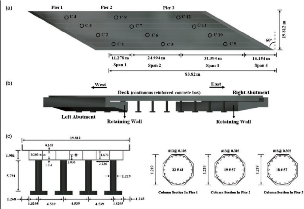
(a) Plan view of all four spans (b) Elevation (c) Column Elevation & Column cross-section
