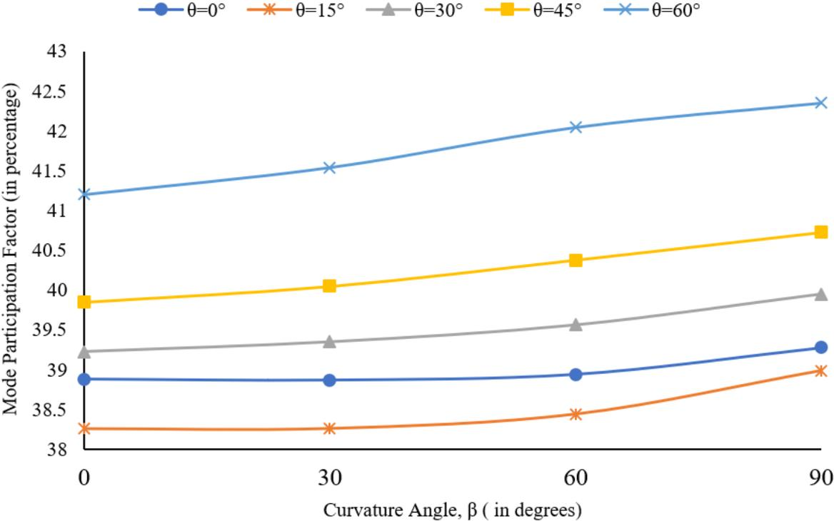
**Figure 4.6.** Mode Participation Factor of first In-Plane Mode for various bridge configurations
