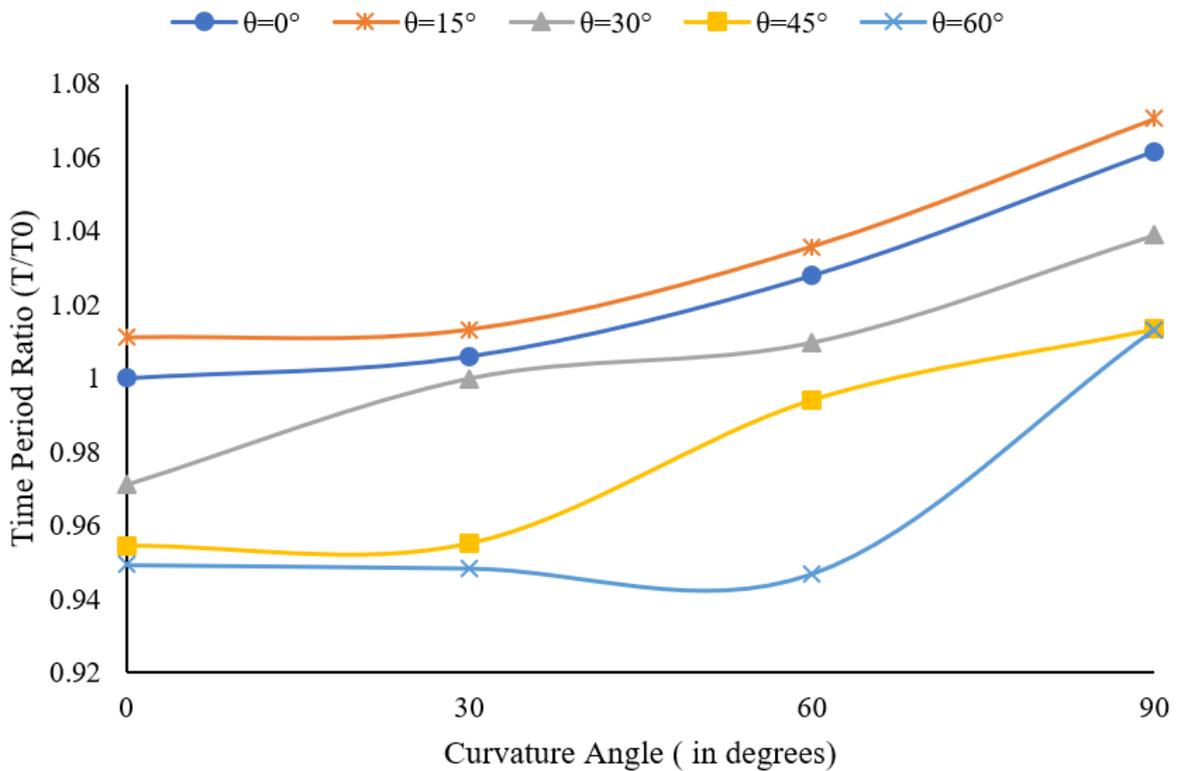
**Figure 4.5.** Time Periods Ratio of 1<sup>st</sup> Out of Plane mode for various bridge configurations
