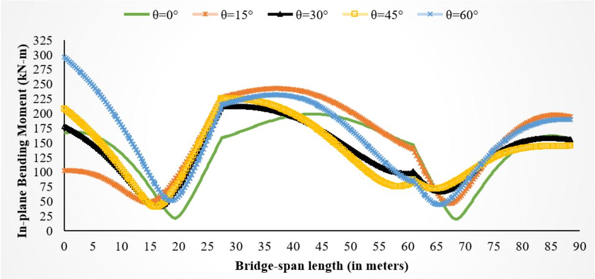
a) In-plane Bending Moment for bridge models having Curvature Angle ( $\beta$ ) of 30° with different Skew Angles under Vertical Excitations
