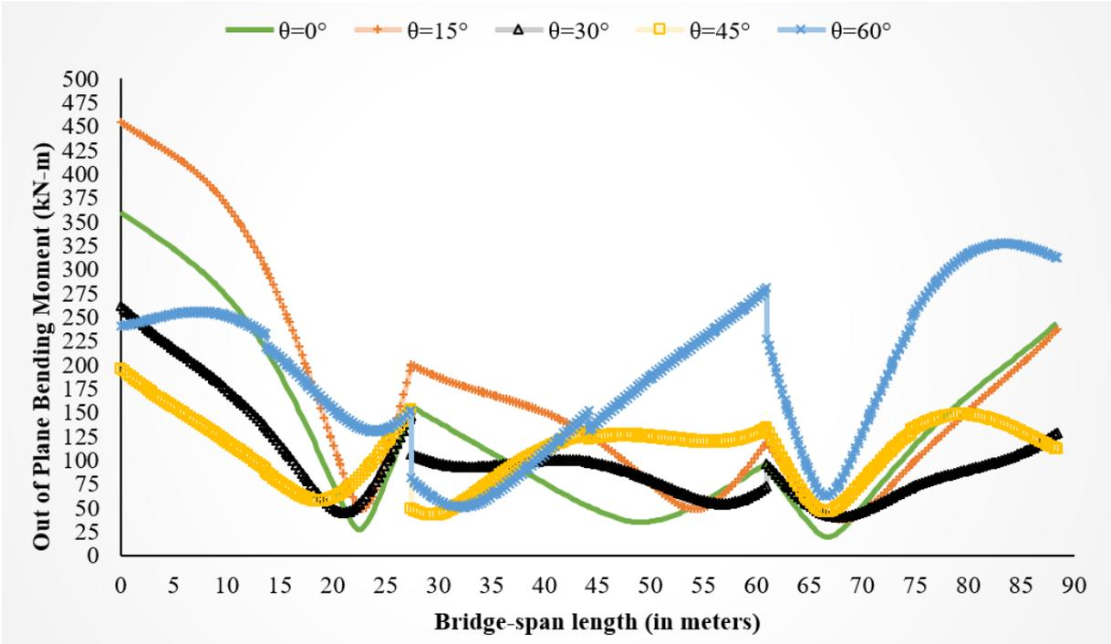
a) Out-of-Plane Bending Moment for bridge models having Curvature Angle ( $\beta$ ) of 30° with different Skew Angles under Longitudinal Excitations
