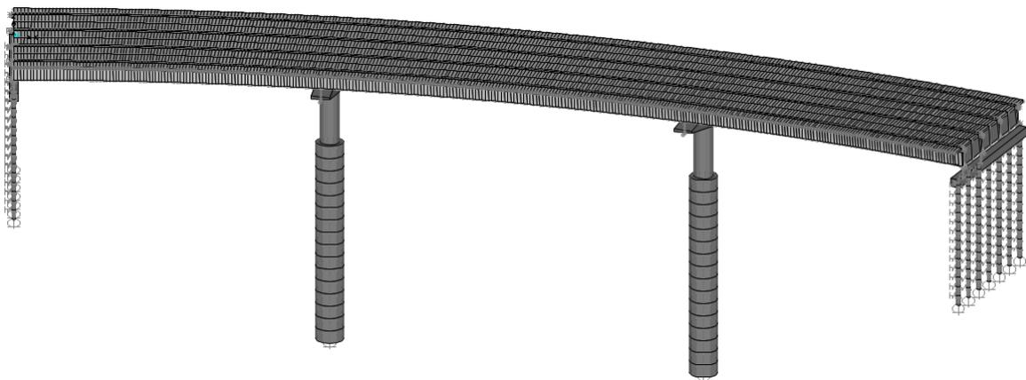
**Figure 3.17** 3-D model of bridge for configuration of  $\beta=30^\circ$  and  $\theta=0^\circ$
