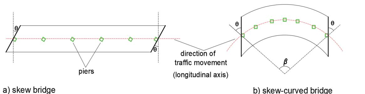
NOTE: position of abutments in case of no skewness is shown by black dotted lines
