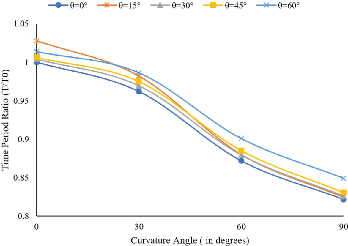
**Figure 4.3.** Time Periods Ratio of 1<sup>st</sup> In-Plane mode for various bridge configurations
