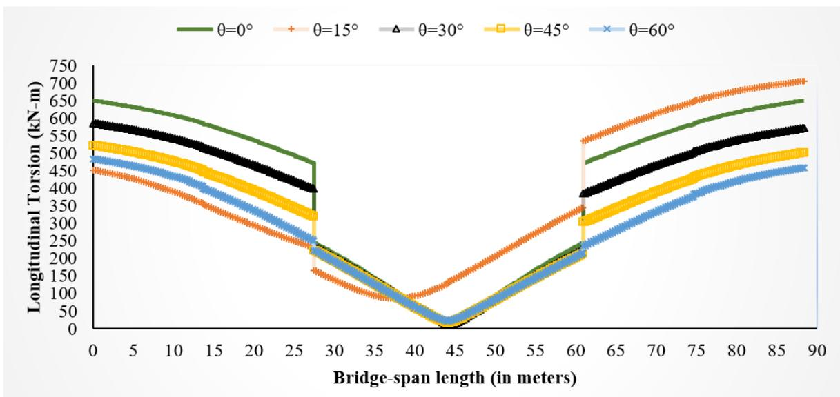
**Figure 5.9** Longitudinal Torsion for bridge models having Curvature Angle ( $\beta$ ) of  $0^\circ$  with different Skew Angles under Transverse Excitations
