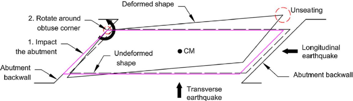
**Figure 2.1** Unseating Mechanism in a typical Skew Bridge during Earthquake [12]
