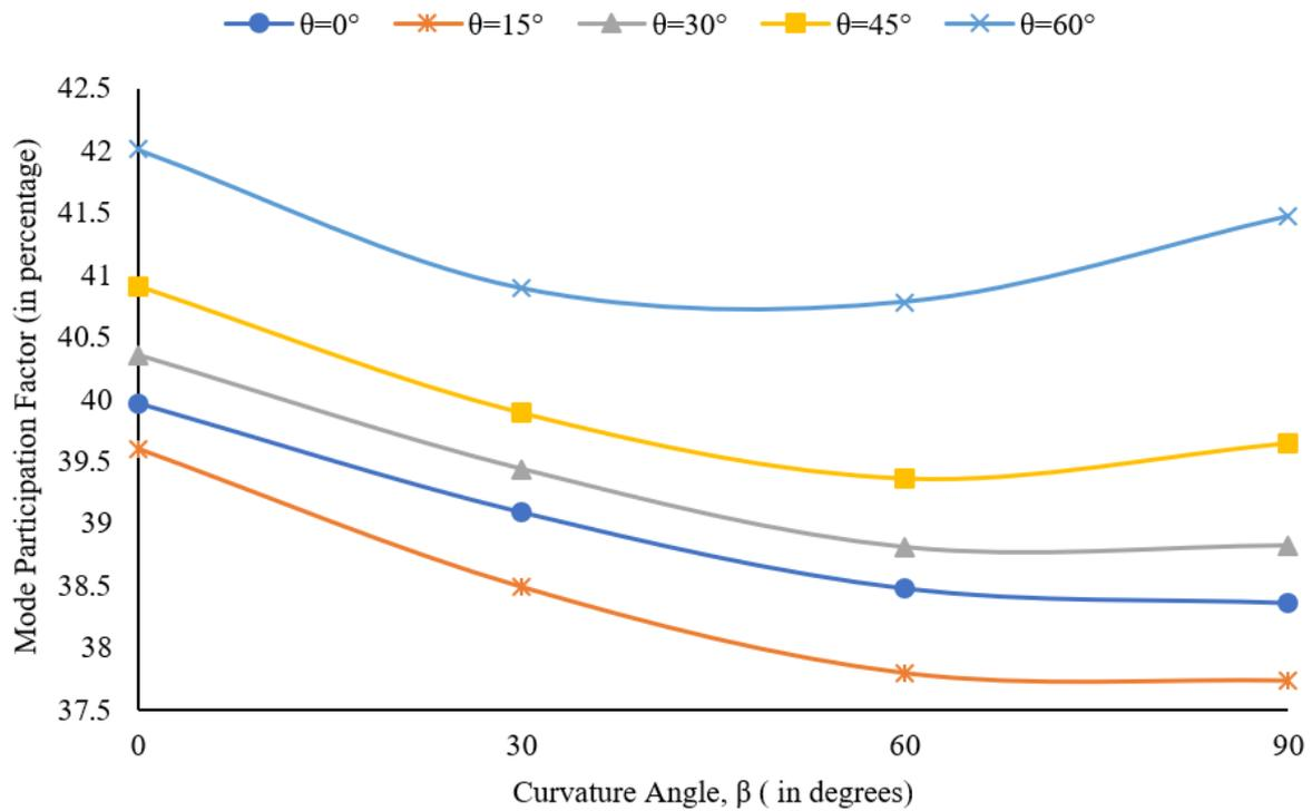
**Figure 4.7.** Mode Participation Factor of first Longitudinal Mode for various bridge configurations
