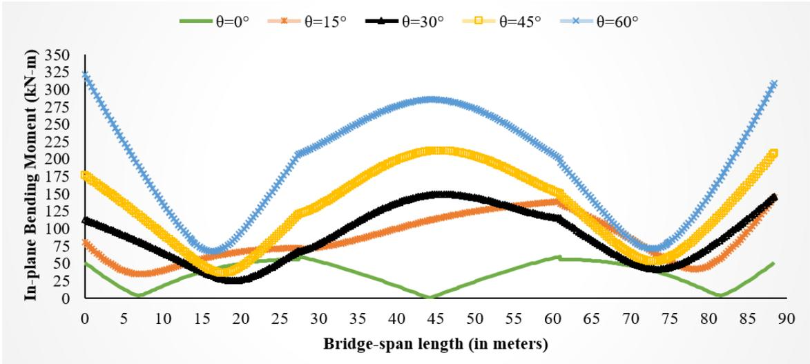
Figure 5.5 In-plane Bending Moment for bridge models having Curvature Angle ( $\beta$ ) of  $0^\circ$  with different Skew Angles under Longitudinal Excitations
