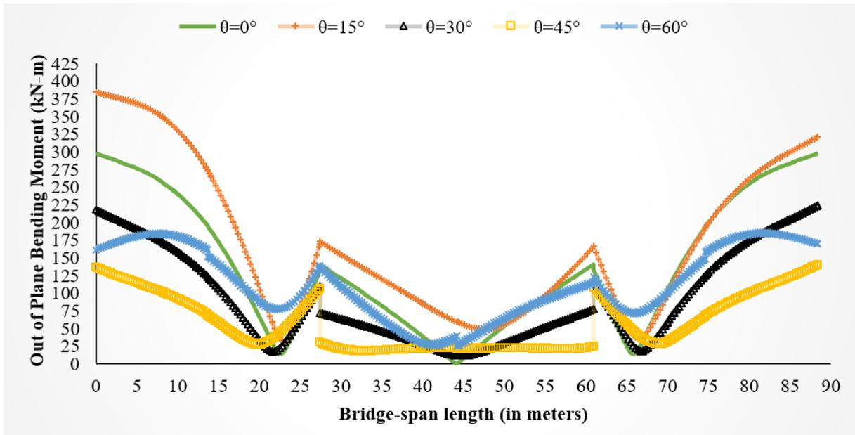
**Figure 5.2** Out-of-Plane Bending Moment for bridge models having Curvature Angle ( $\beta$ ) of  $0^\circ$  with different Skew Angles under Longitudinal Excitations
