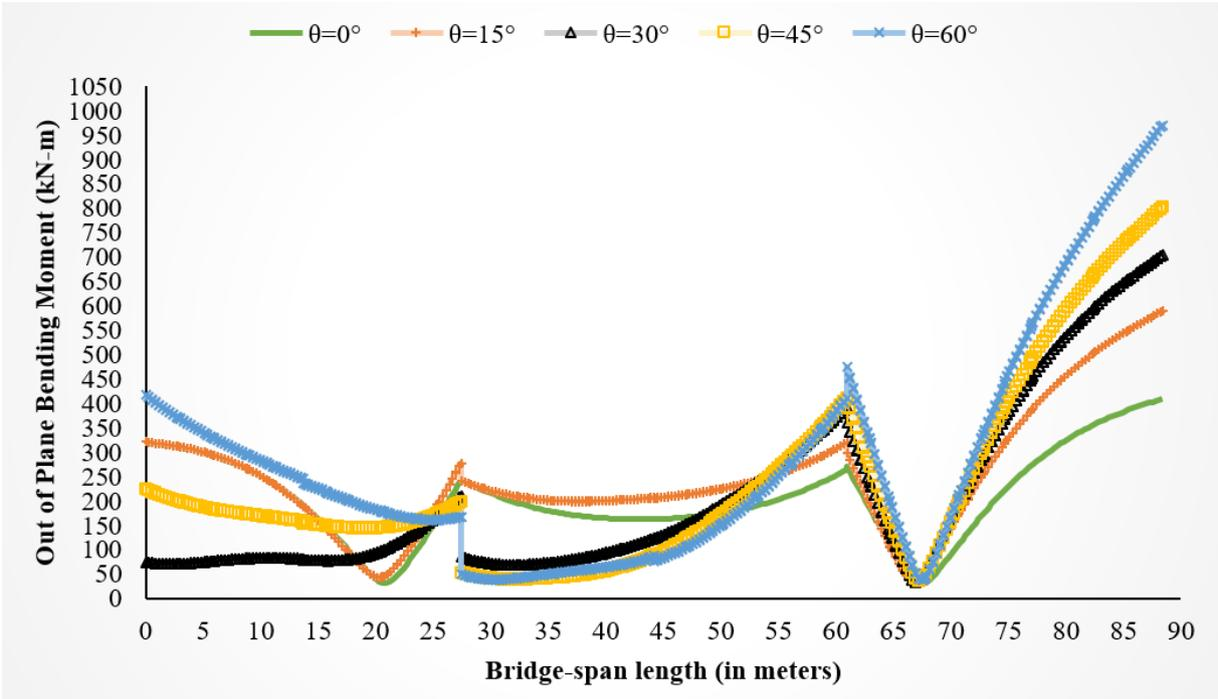
a) Out-of-Plane Bending Moment for bridge models having Curvature Angle ( $\beta$ ) of 30° with different Skew Angles under Transverse Excitations
