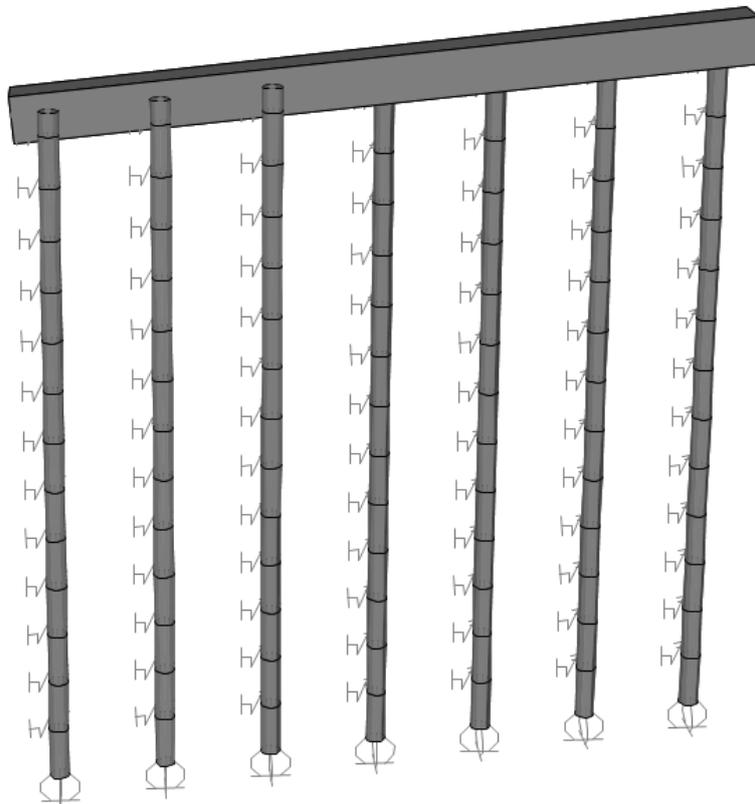
Figure 3.12 Modelling Details of 13 soil springs used for accounting the behaviour of lateral stiffness of the soil. Same soil properties of the soil have been used as that of the pier shaft. Abutment piles have been provided in group, therefore modulus of subgrade reaction of 0.7 has been used. Discrete
