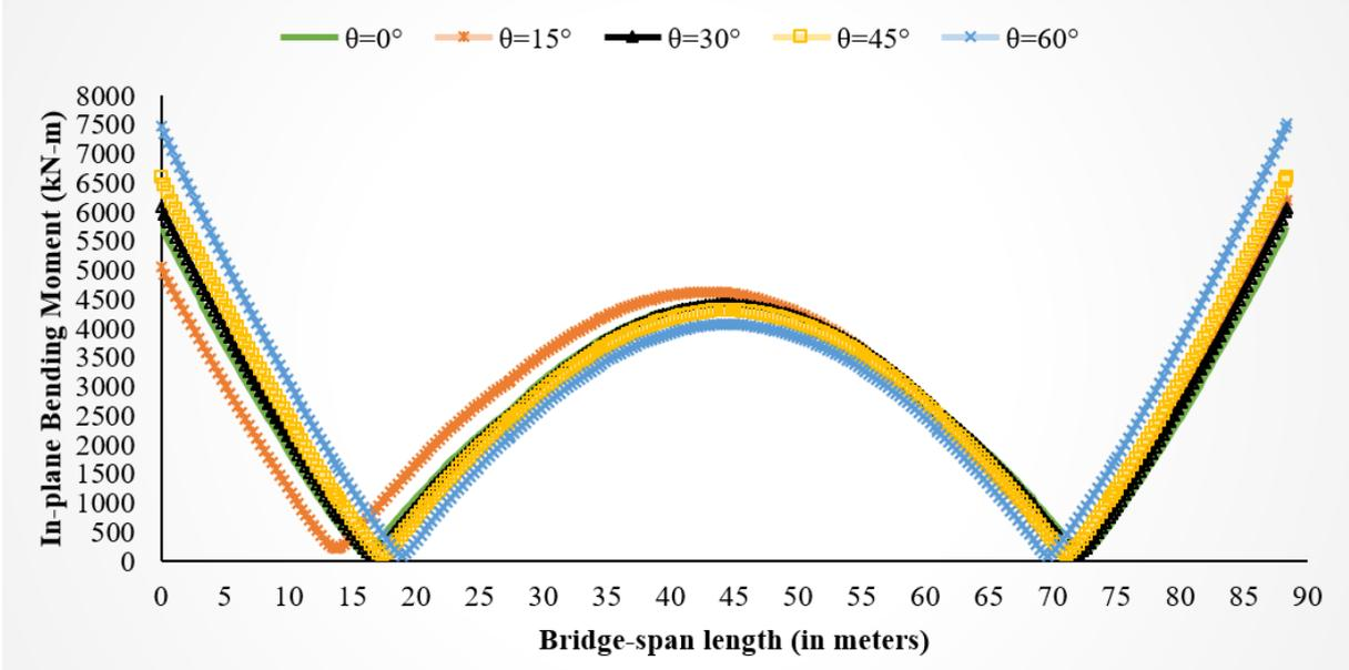
**Figure 5.6** In-plane Bending Moment for bridge models having Curvature Angle ( $\beta$ ) of  $0^\circ$  with different Skew Angles under Transverse Excitations
