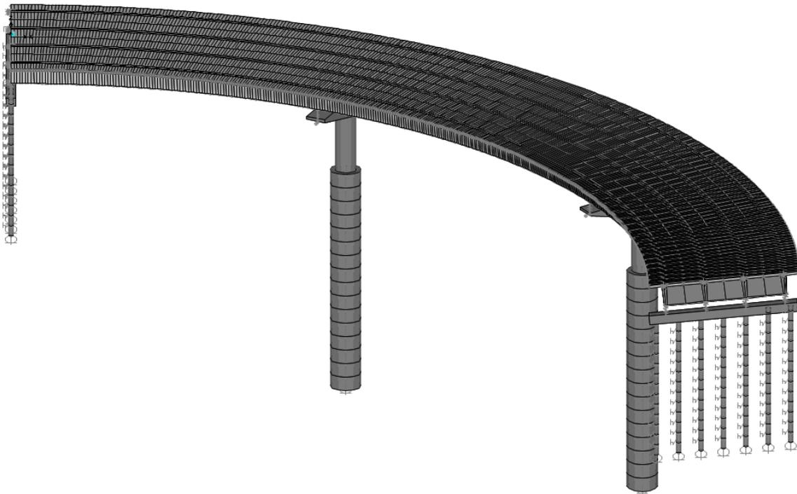
**Figure 3.21** 3-D model of bridge for configuration of  $\beta=90^\circ$  and  $\theta=0^\circ$
