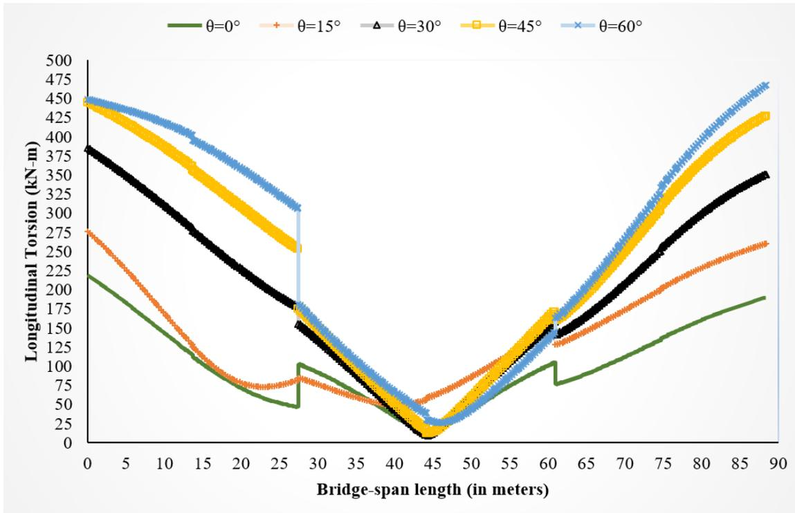
b) Longitudinal Torsion for bridge models having Curvature Angle ( $\beta$ ) of  $60^\circ$  with different Skew Angles under Longitudinal Excitations
