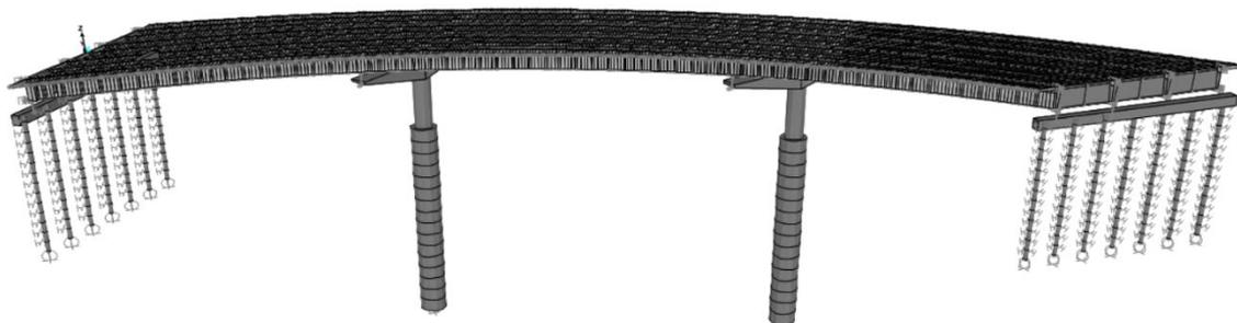
**Figure 3.8** 3-D model for bridge configuration having curvature angle,  $\beta=60^\circ$  and skew angle,  $\theta=45^\circ$
