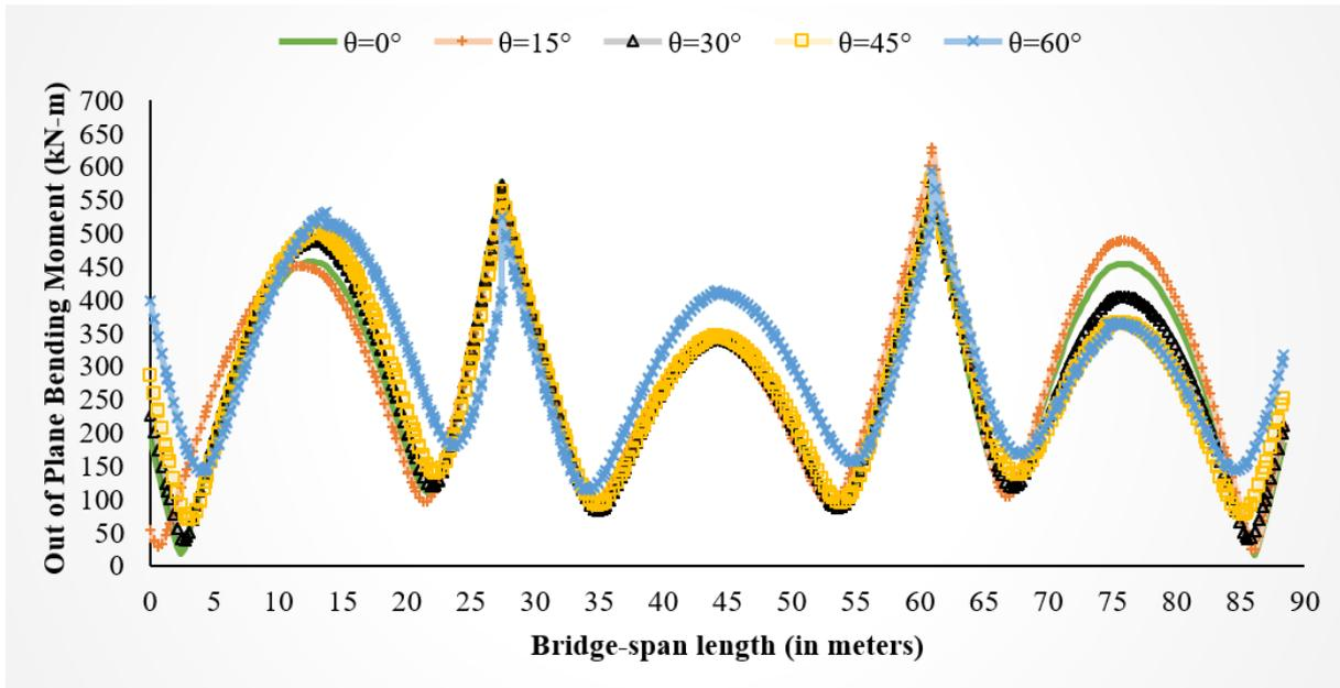
b) Out-of-Plane Bending Moment for bridge models having Curvature Angle ( $\beta$ ) of  $60^\circ$  with different Skew Angles under Vertical Excitations
