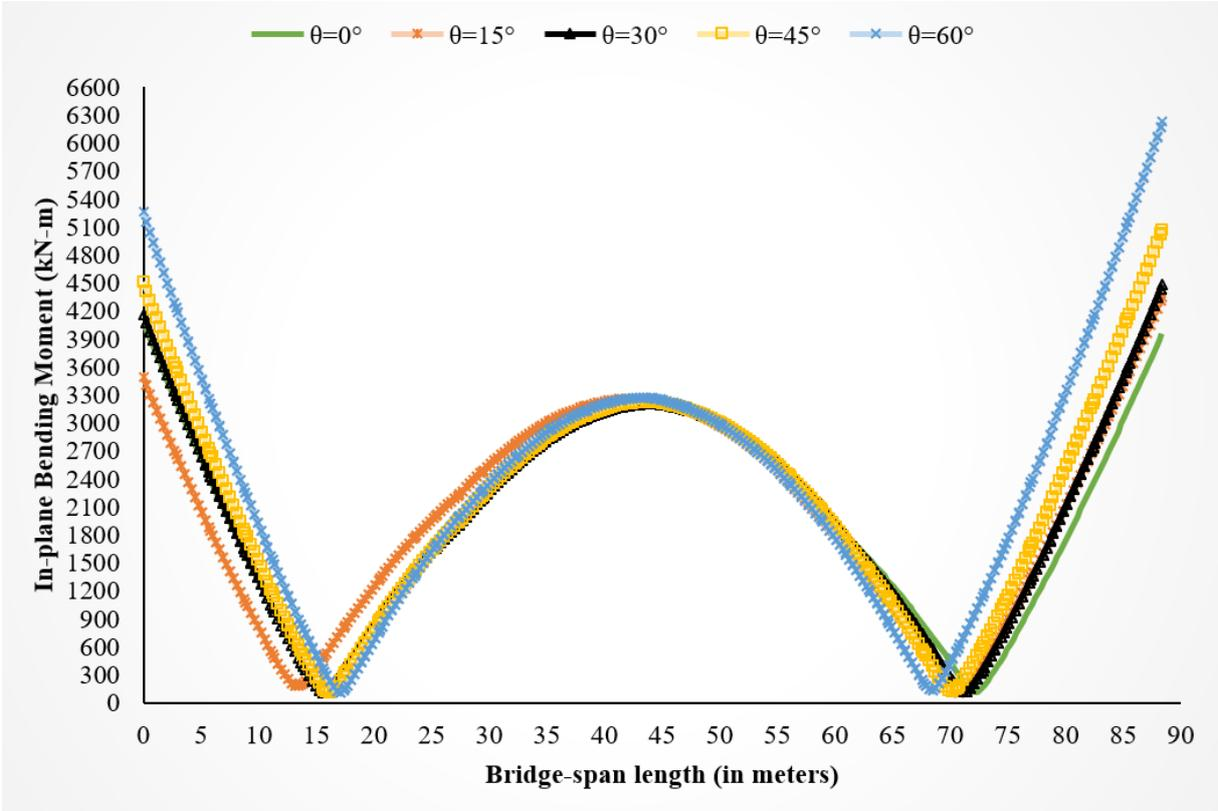
a) In-plane Bending Moment for bridge models having Curvature Angle ( $\beta$ ) of  $30^\circ$  with different Skew Angles under Transverse Excitations
