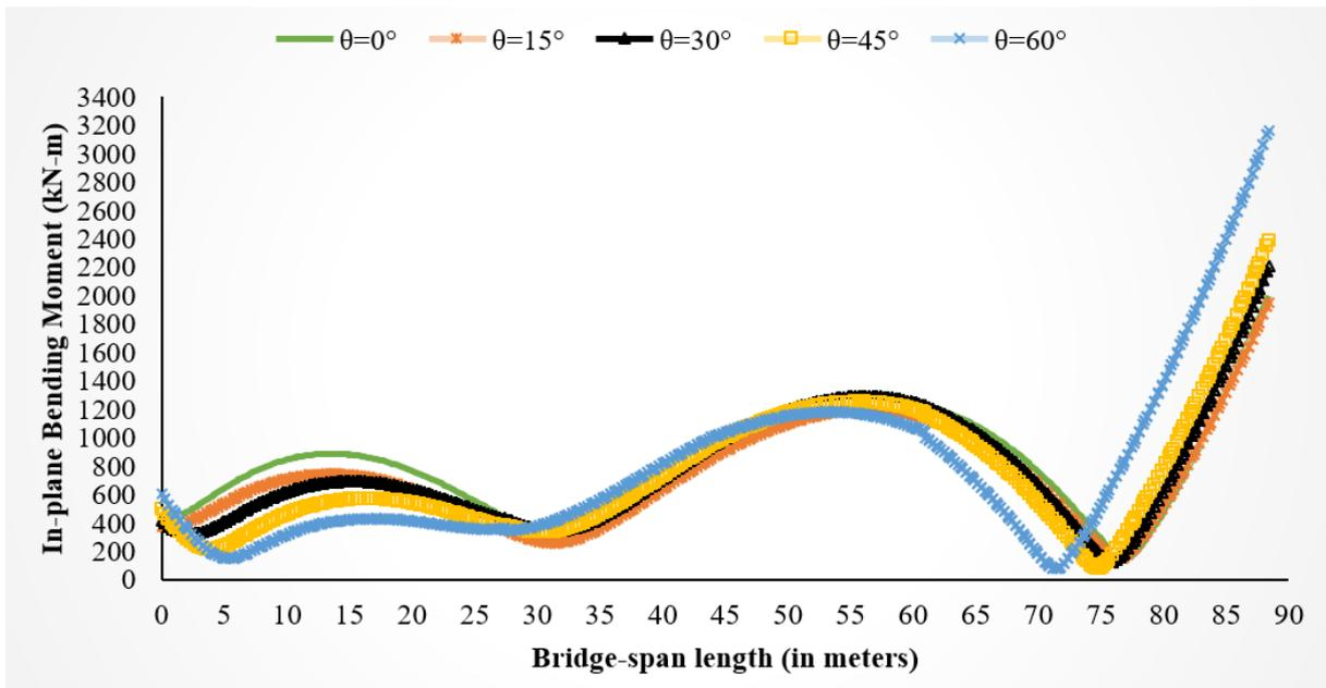
c) In-plane Bending Moment for bridge models having Curvature Angle ( $\beta$ ) of  $90^\circ$  with different Skew Angles under Longitudinal Excitations
