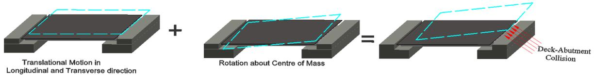
**Figure 2.4** Seismic Pounding due to Deck-Abutment Collision
