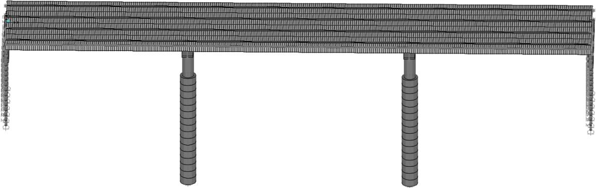
**Figure 3.15** 3-D model of bridge for configuration of  $\beta=0^\circ$  and  $\theta=0^\circ$  i.e. a straight bridge configuration
