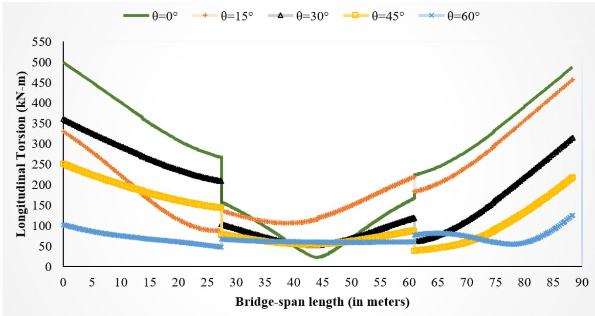
b) Longitudinal Torsion for bridge models having Curvature Angle ( $\beta$ ) of  $60^\circ$  with different Skew Angles under Transverse Excitations
