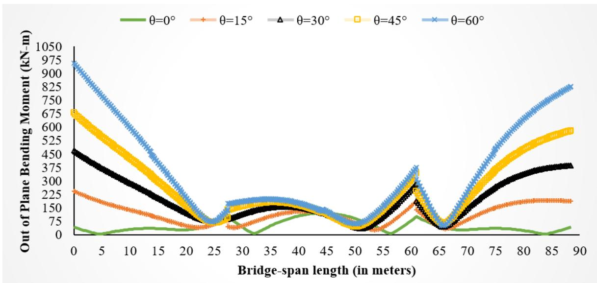
**Figure 5.3** Out-of-Plane Bending Moment for bridge models having Curvature Angle ( $\beta$ ) of  $0^\circ$  with different Skew Angles under Transverse Excitations
