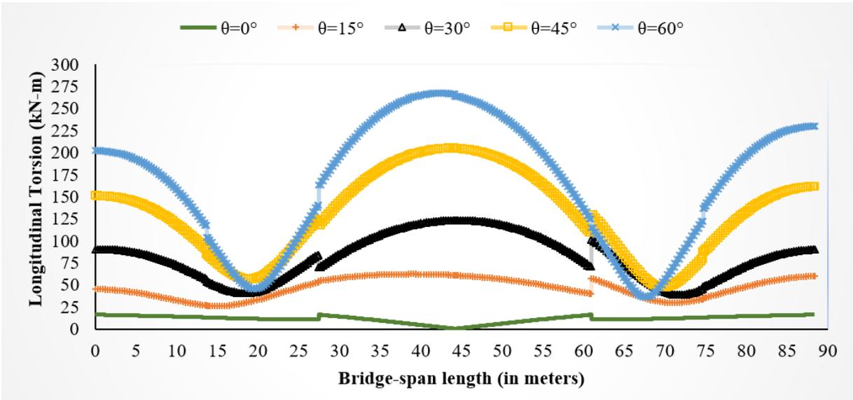
**Figure 5.10** Longitudinal Torsion for bridge models having Curvature Angle ( $\beta$ ) of  $0^\circ$  with different Skew Angles under Vertical Excitations
