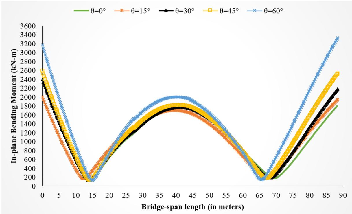
b) In-plane Bending Moment for bridge models having Curvature Angle ( $\beta$ ) of  $60^\circ$  with different Skew Angles under Transverse Excitations
