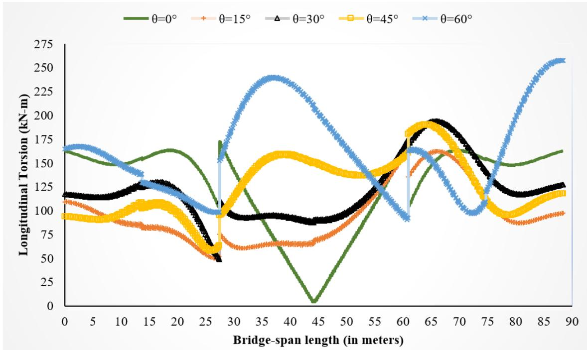
c) Longitudinal Torsion for bridge models having Curvature Angle ( $\beta$ ) of  $90^\circ$  with different Skew Angles under Vertical Excitations
