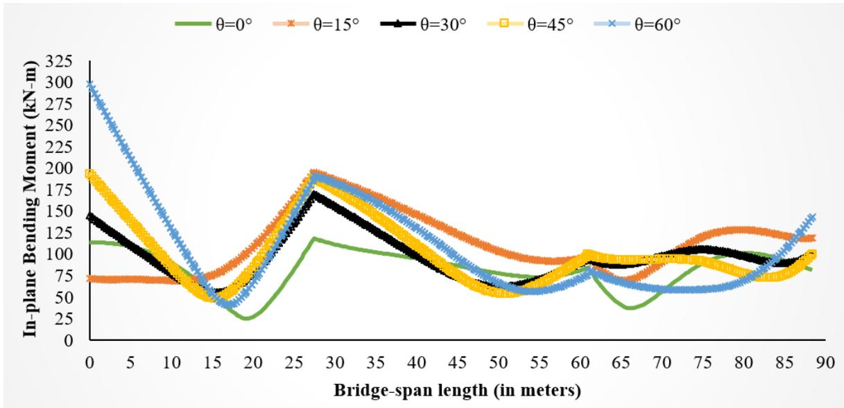
b) In-plane Bending Moment for bridge models having Curvature Angle ( $\beta$ ) of  $60^\circ$  with different Skew Angles under Vertical Excitations
