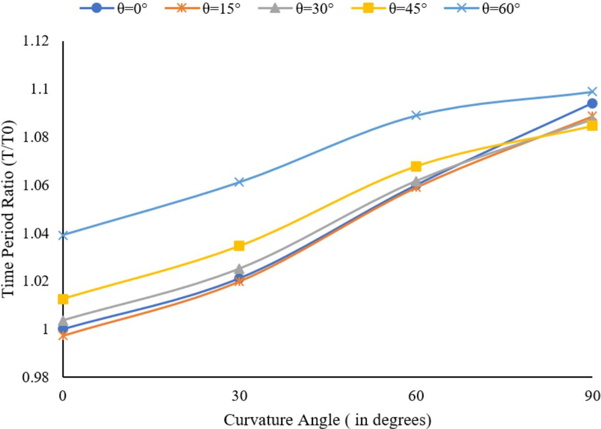
**Figure 4.4.** Time Periods Ratio of 1<sup>st</sup> Longitudinal mode for various bridge configurations
