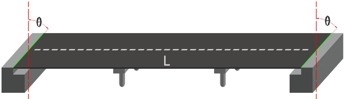
Figure 1.3 Skew Bridge Geometry
