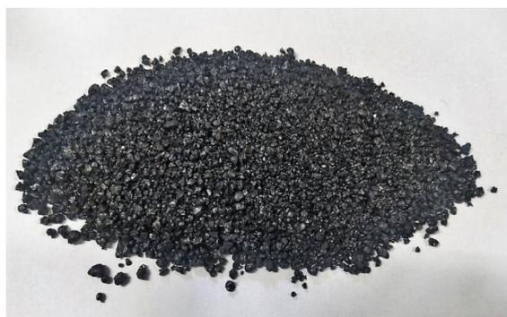
**Fig: 3.3** Copper Slag.
