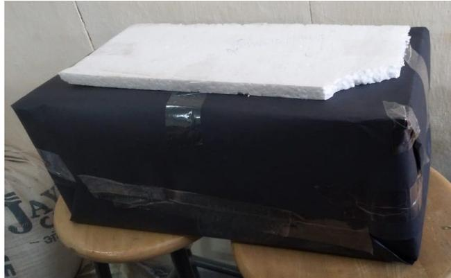
**Fig: 3.8** Control dark chamber for testing of sample in controlled condition.
