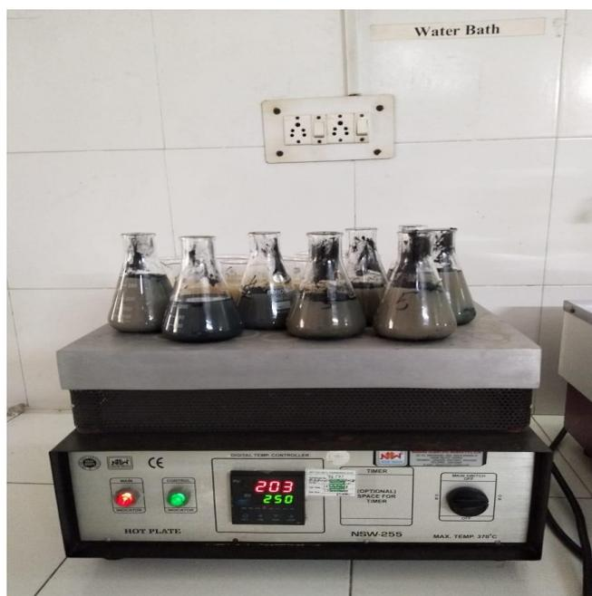
**Fig: 3.30** Digestion of phosphorus.
