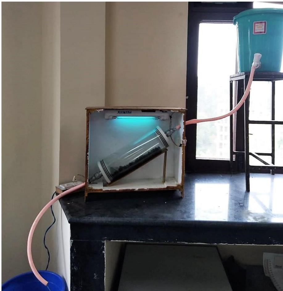
**Fig: 3.22** Laboratory image for UV+ $\text{H}_2\text{O}_2$ + $\text{TiO}_2$  Degradation.
