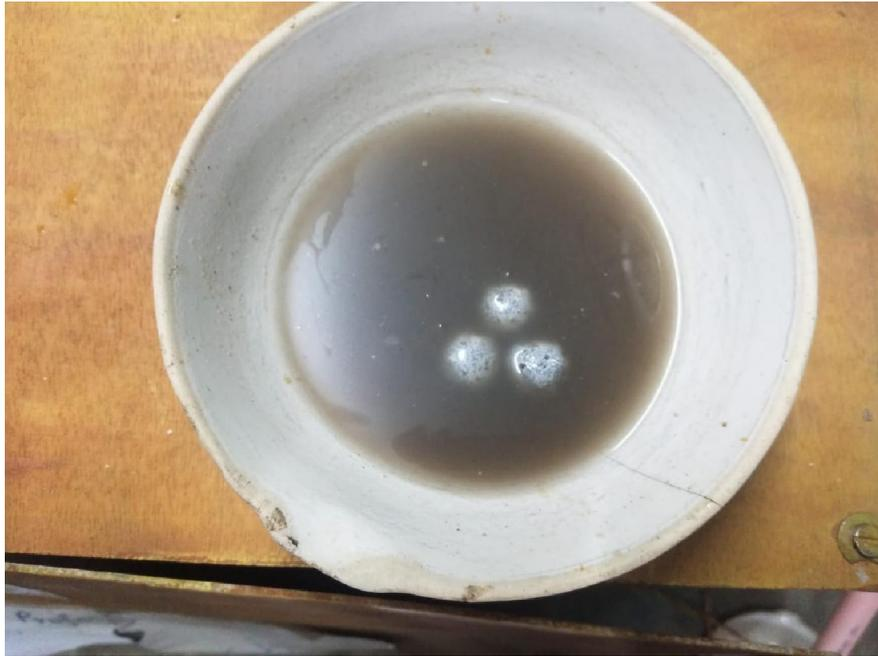
**Fig: 3.16** Copper pellets coated with  $\text{TiO}_2$  dipped in greywater.
