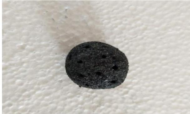
**Fig: 3.13** Formation of holes in pellet.
