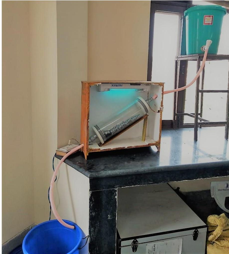
**Fig: 3.24** Laboratory image for UV+H<sub>2</sub>O<sub>2</sub>+TiO<sub>2</sub>+Fe Degradation.
