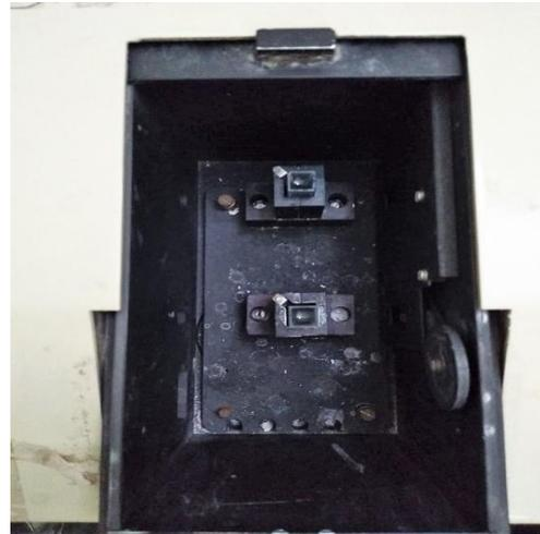
Fig: 3.28 Turbidity measuring using Spectrometer.
