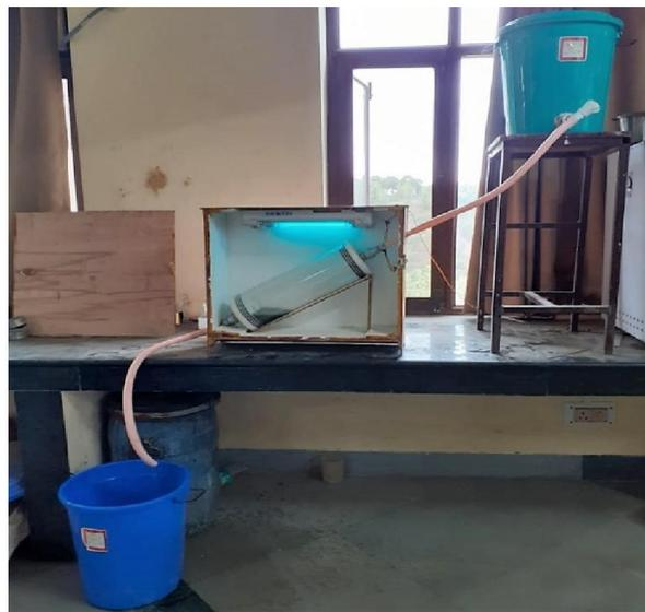
**Fig: 3.18** Laboratory Image for Only UV Degradation
