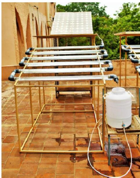
**Fig: 2.9** Tubular Slurry type Ag – TiO<sub>2</sub> photoreactor [49]
