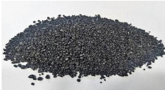
**Fig: 3.11** Copper slag for grinding.
