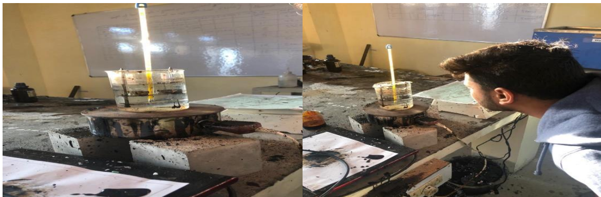
Fig. 4.6 Softening point test apparatus
