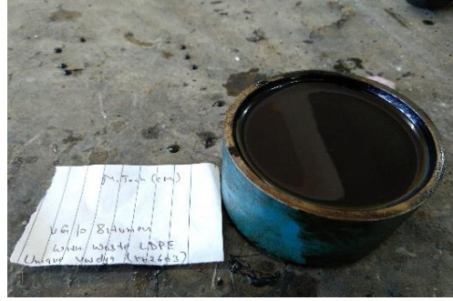
Fig. 4.2 Sample for penetration test
