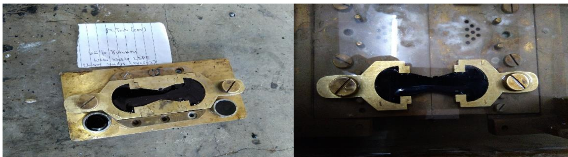
Fig. 4.4 Ductility test sample
