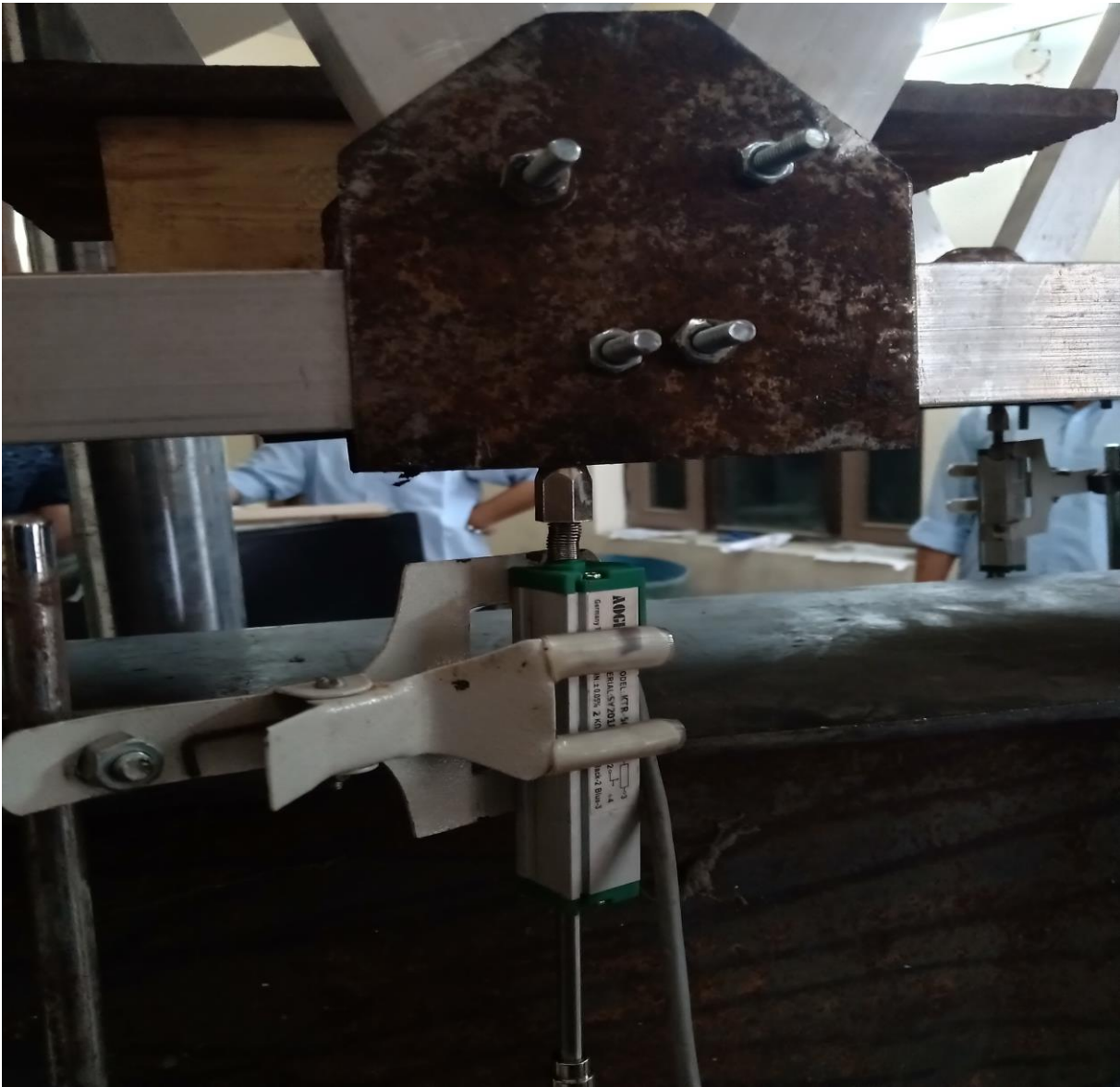
Figure 3.21 Image of Linear Variable Differential Transformer attached to node.
