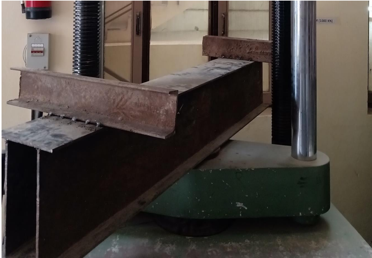
Fig. 3.25 Image of Support system in UTM
