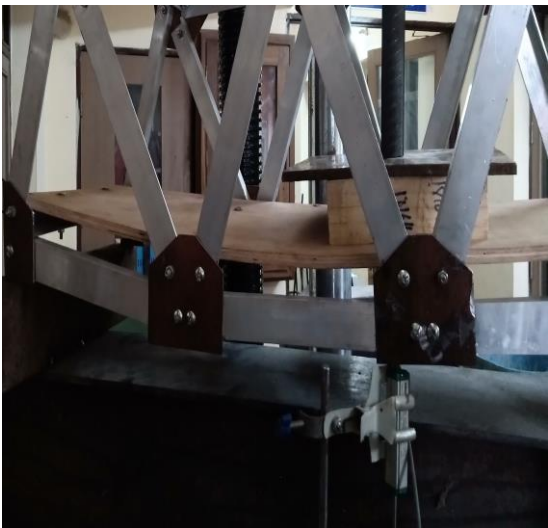
Fig. 4.12 Deformation in Angle section after testing
