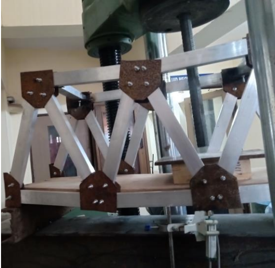
Fig. 4.13 Deformation in Hollow section after testing
