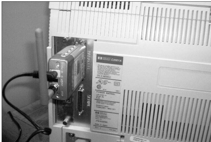
Figure 6-4: Wireless print server attached to a printer.
